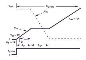
Figure 18. Gate Charge Waveforms
