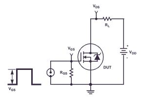
Figure 19. Switching Time Test Circuit
