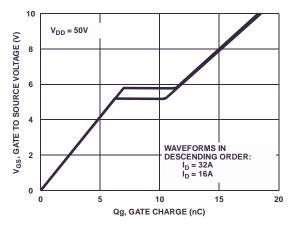
Figure 14. Gate Charge Waveforms for Constant Gate Currents
