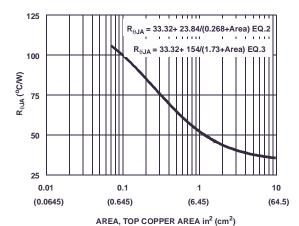
Figure 21. Thermal Resistance vs Mounting
