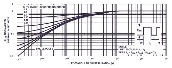
Figure 3. Normalized Maximum Transient Thermal Impedance
