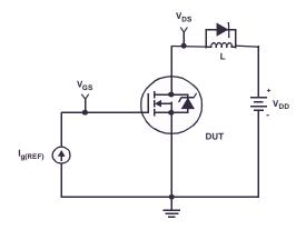
Figure 17. Gate Charge Test Circuit
