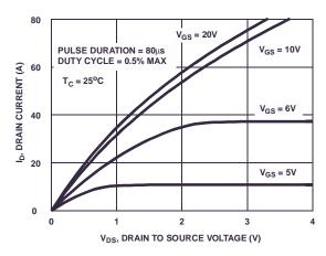
Figure 7. Transfer Characteristics
