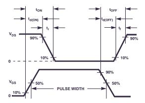
Figure 20. Switching Time Waveforms
