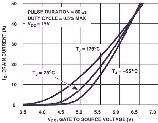
Figure 7. Transfer Characteristics
