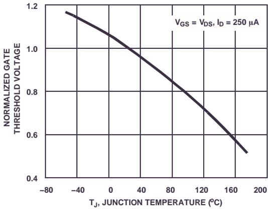
Figure 11. Normalized Gate Threshold vs. Junction Temperature
