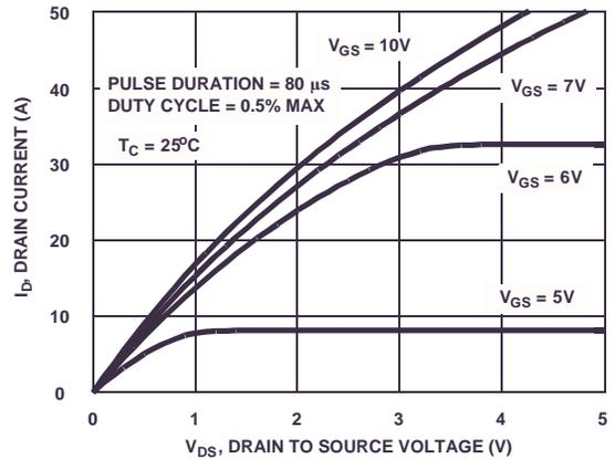
Figure 8. Saturation Characteristics
