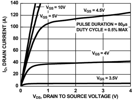
Figure 8. Saturation Characteristics
