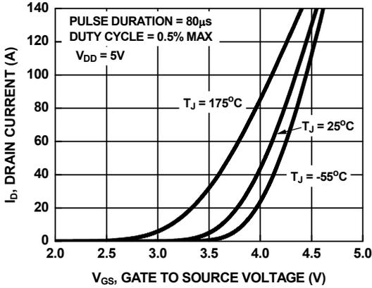
Figure 7. Transfer Characteristics
