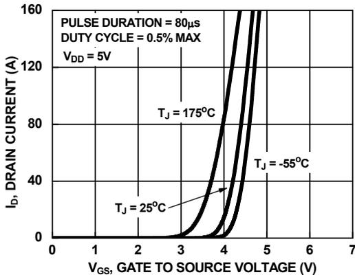
Figure 7. Transfer Characteristics
