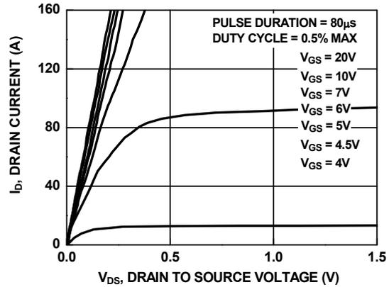
Figure 8. Saturation Characteristics
