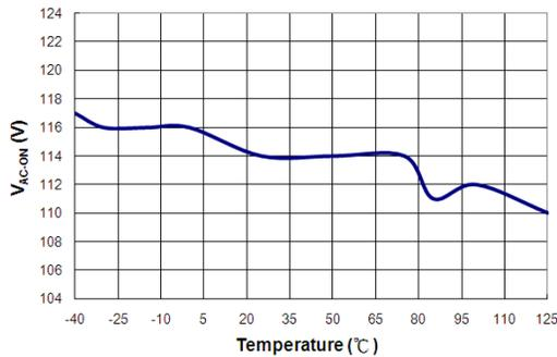
**Figure 23. Brownin (V<sub>AC-ON</sub>) vs. Temperature**
