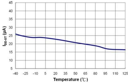
Figure 9. Startup Current ( $I_{DD-ST}$ ) vs. Temperature
