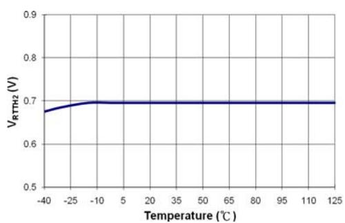
**Figure 22. Over-Temperature Protection Threshold Voltage (V<sub>RTTH2</sub>) vs. Temperature**
