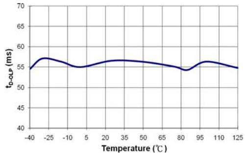
**Figure 18. Delay Time of FB Pin Open-Loop Protection (t<sub>D-OLP</sub>) vs. Temperature**
