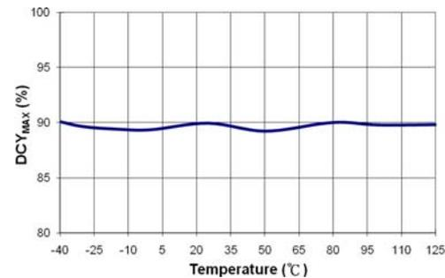
Figure 16. Maximum Duty Cycle ( $DCY_{MAX}$ ) vs. Temperature
