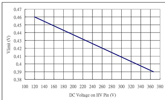
Figure 25. Linearly Current Limit Curve
