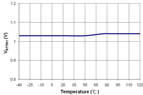
**Figure 21. Over-Temperature Protection Threshold Voltage (V<sub>RTTH1</sub>) vs. Temperature**
