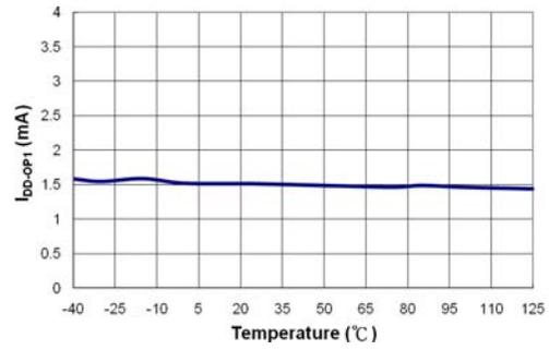
Figure 10. Operation Supply Current ( $I_{DD-OP1}$ ) vs. Temperature
