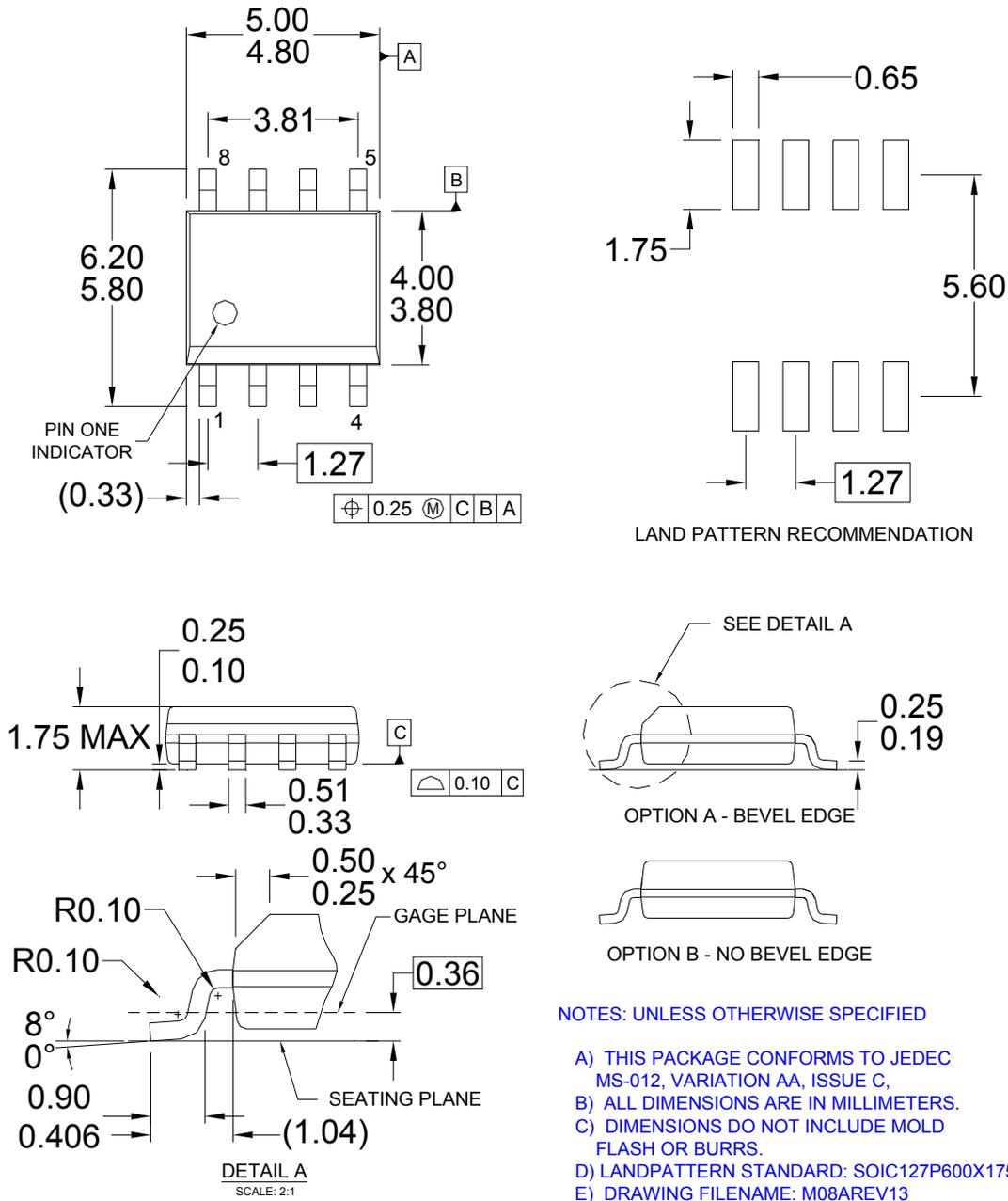
**Figure 26. 8-Pin, Small Outline Package (SOP) Package**
