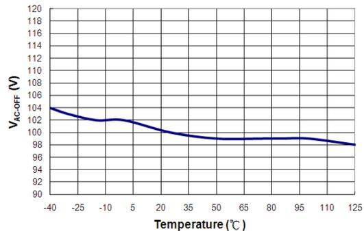
**Figure 24. Brownout (V<sub>AC-OFF</sub>) vs. Temperature**
