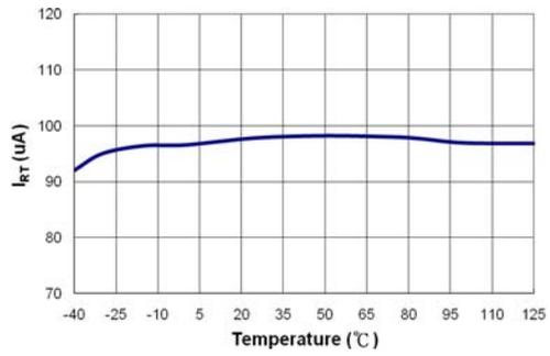
**Figure 20. Output Current from RT Pin (I<sub>RT</sub>) vs. Temperature**
