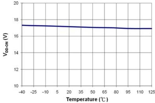
Figure 11. Start Threshold Voltage ( $V_{DD-ON}$ ) vs. Temperature
