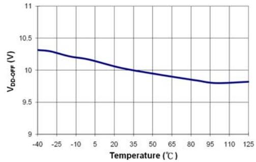
Figure 12. Minimum Operating Voltage ( $V_{DD-OFF}$ ) vs. Temperature
