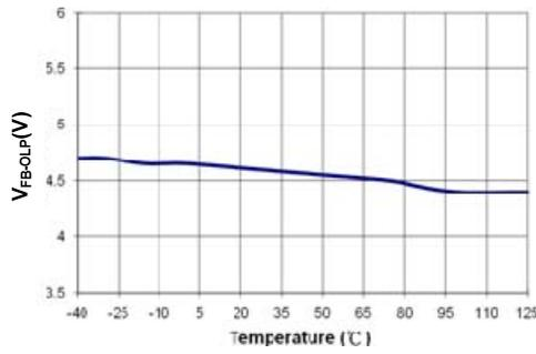
**Figure 17. FB Open-Loop Trigger Level (V<sub>FB-OLP</sub>) vs. Temperature**
