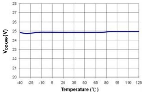
**Figure 19. V<sub>DD</sub> Over-Voltage Protection (V<sub>DD-OVP</sub>) vs. Temperature**
