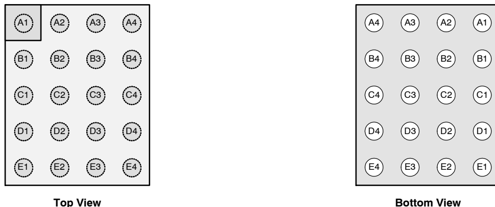
Figure 3. WLCSP-20 Pin Assignments
