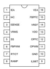
Figure 6. Pin Configuration (Top View)
