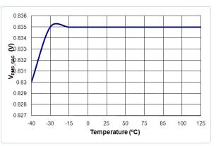
Figure 24. V<sub>RMS-SAG</sub> vs. Temperature
