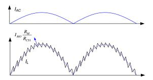
Figure 33. Inductor Current Shaping
