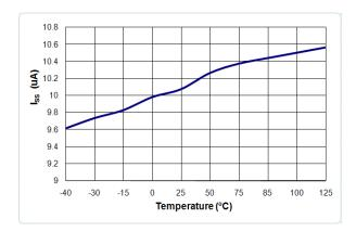
Figure 23. Iss vs. Temperature
