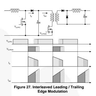
Figure 27 shows the interleaved leading / trailing edge modulation, where the turn-off of the PFC drive signal is synchronized to the turn-on of the PWM drive signal. This technique allows the PFC output diode current to flow directly into the downstream DC/DC converter, minimizing the current ripple of PFC output capacitor.
