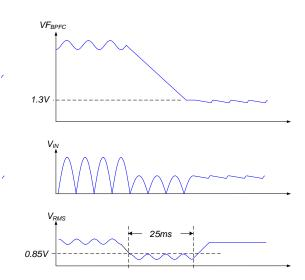
Figure 38. The Second condition of Sag Protection
