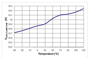
Figure 20. V<sub>GATE-CLAMP-PWM</sub> vs. Temperature
