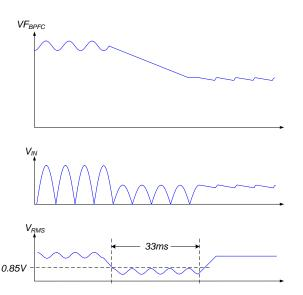
Figure 37. The First Condition of Sag Protection
