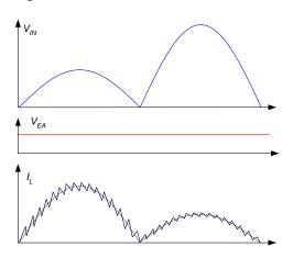
Figure 30. Line Feed-Forward Operation
