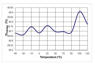
Figure 22. D<sub>PWM-MAX</sub> vs. Temperature
