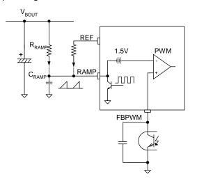
Figure 35. PWM Ramp Generation Circuit
