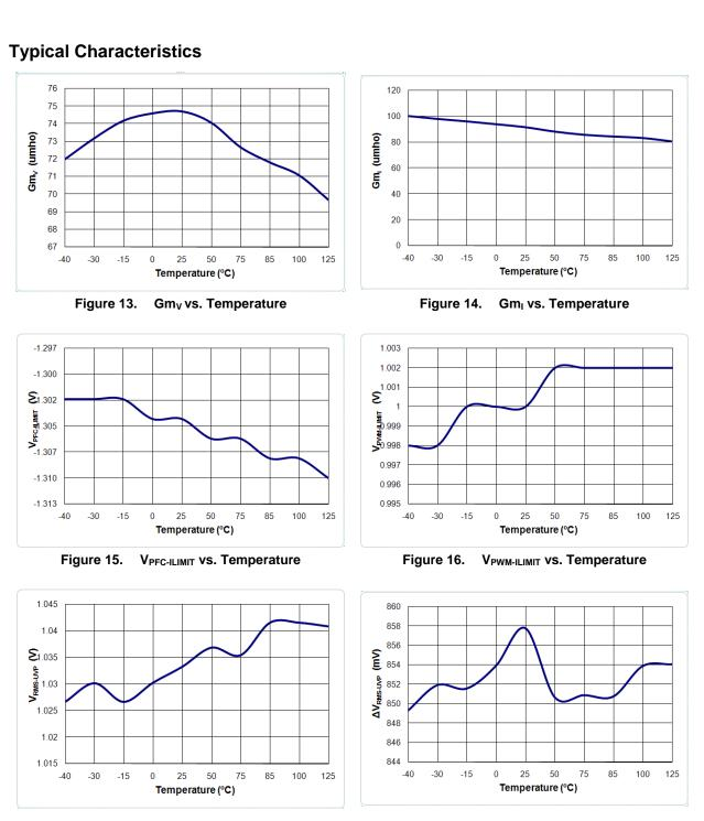
Figure 17. V<sub>RMS-UVP</sub> vs. Temperature
