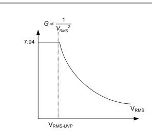
Figure 29. Modulation Gain Characteristics
