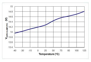
Figure 19. V<sub>GATE-CLAMP-PFC</sub> vs. Temperature
