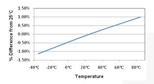
Figure 12. Shunt Regulator Voltage vs. Temperature
