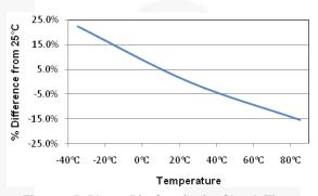
Figure 15. Phase Pin Continuity Check Time vs. Temperature
