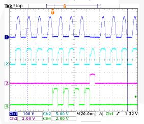
Figure 9. GFI / Sense Coil Tests Ch1: SCR Anode (100 V/div), Ch2: Phase (Pin 4), Ch3: EOL Alarm (Pin 5), Ch4: Fault Test (Pin 6)<sup>(10)</sup>
