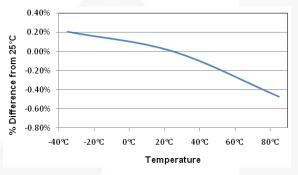
Figure 14. Under-Voltage Reset vs. Temperature
