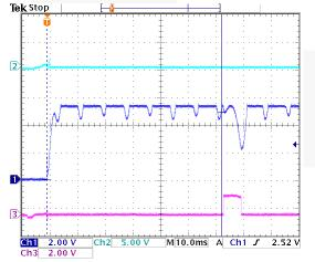
Figure 11. Phase Pin, Continuity Test; Ch1: VDD (Pin 3), Ch2: Phase (Pin 4), Ch3: EOL Alarm (Pin 5)<sup>(12,13)</sup>
