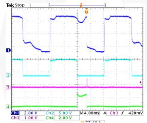
Figure 6. Pass Simulated Ground Fault Test; Ch1: SCR Test (Pin 1), Ch2: Phase (Pin 4), Ch3: SCR Gate, Ch4: Fault Test (Pin 6)<sup>(7)</sup>
