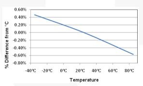
Figure 16. Phase Pin Voltage Clamp High vs. Temperature
