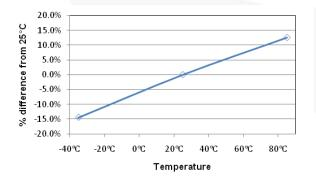
Figure 18. Fault Test Pin Current vs. Temperature
