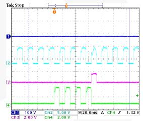
Figure 10. Solenoid Test Ch1: SCR Anode (100 V/Div), Ch2: Phase (Pin 4), Ch3: EOL Alarm (Pin 5), Ch4: Fault Test (Pin 6)<sup>(11)</sup>
