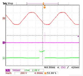
Figure 4. Pass GFCI, Sense Coil, Solenoid, SCR Tests; Ch Math: V<sub>AC</sub> Input 200 V/Div, Ch3: SCR Gate, Ch4: Fault Test (Pin 6)<sup>(6)</sup>
