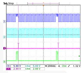
Figure 8. SCR Test Ch1: SCR Test (Pin 1); Ch2: Phase (Pin 4); Ch3: EOL Alarm (Pin 5), Ch4: Fault Test (Pin 6)<sup>(9)</sup>
