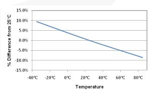
Figure 19. EOL Alarm Pin IOUT vs. Temperature
