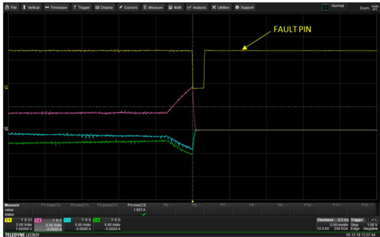
Figure 19. Reaction of Over-current Protection – Detail
