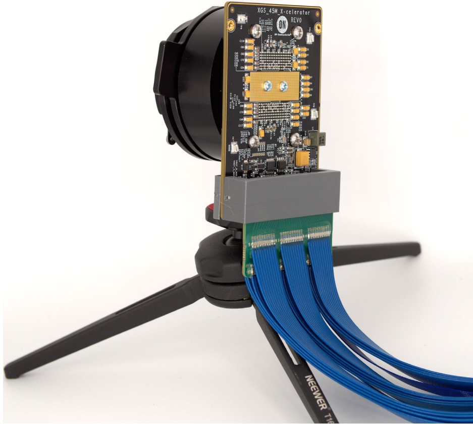
Figure 10. XGS 45000 Development Kit Setup
