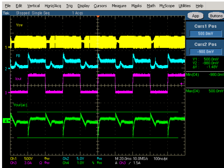
Figure 53. 115 Vac 20 Vout Transient
