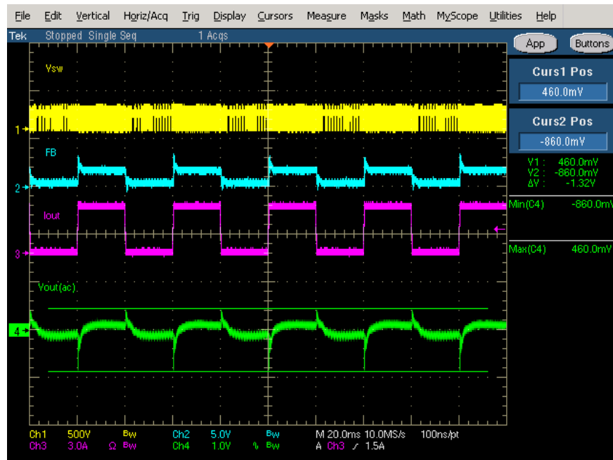
Figure 45. 115 Vac 9 Vout Transient
