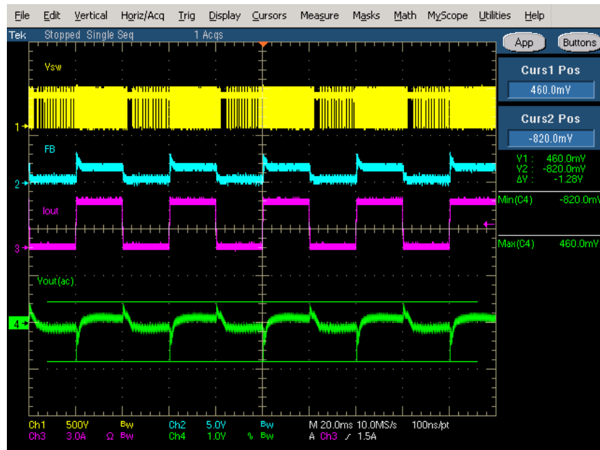
Figure 47. 230 Vac 9 Vout Transient
