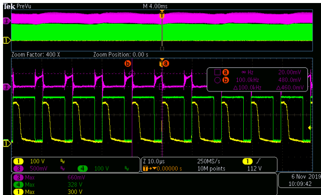
Figure 15. 230 Vac Input, 12 V 25 A Output (CH1 – Low Side Vdrain, CH3 – Current Sense, CH4 – High Side Vdrain)
