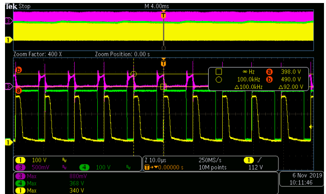
Figure 16. 264 Vac Input, 12 V 25 A Output (CH1 – Low Side Vdrain, CH3 – Current Sense, CH4 – High Side Vdrain)
