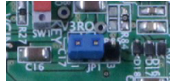
Figure 14. Jumper Switch JP1
