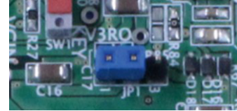
Figure 10. Jumper Switch JP1
