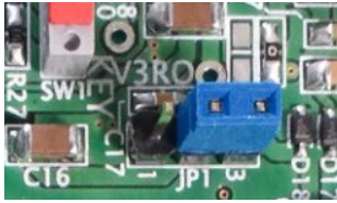
Figure 12. Jumper Switch JP1
