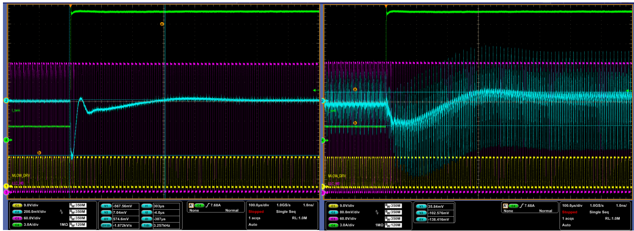
Figure 15. Step Load Response 20 A to 2 A – 50 A/s (Right Measured without Post Inductor)
