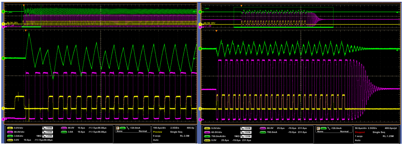
CH1 – LLC Low Side MOSFET Gate-Drive Voltage CH2 – N/A CH3 – LLC HB Node Voltage CH4 – Resonant tank current
