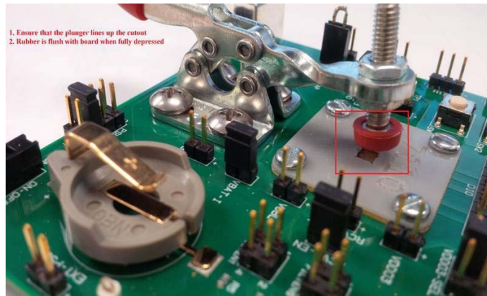
Figure 2. Aligning the Clamp with the Adaptor Plate
