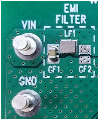
Figure 5. LC Filter on VIN Line
