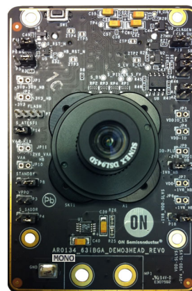
Figure 1. AR0134CS Evaluation Board
