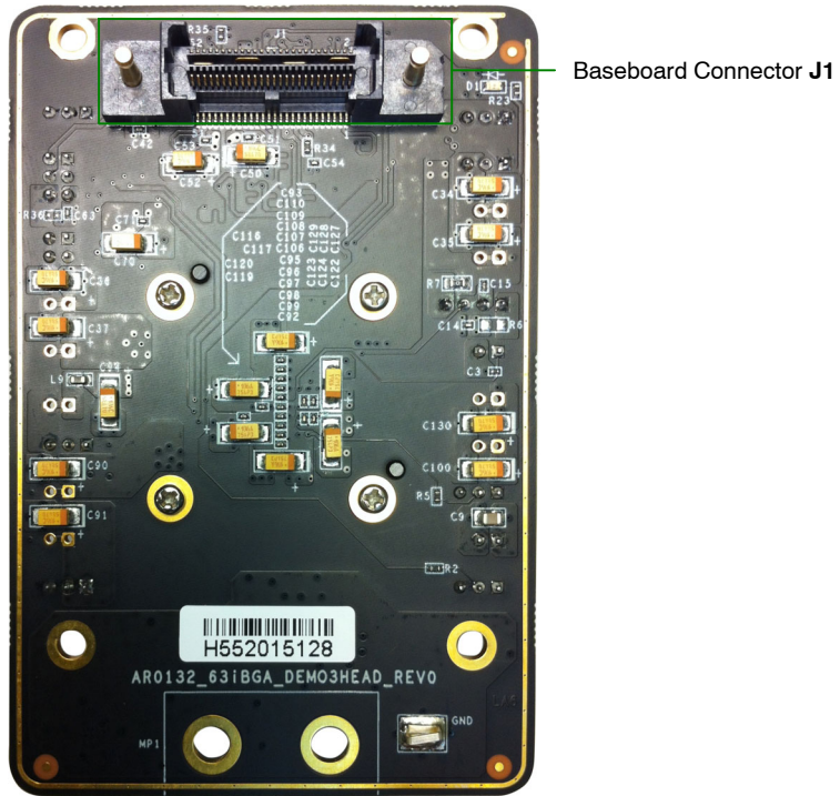
Figure 4. Bottom View of the Board – Connector
