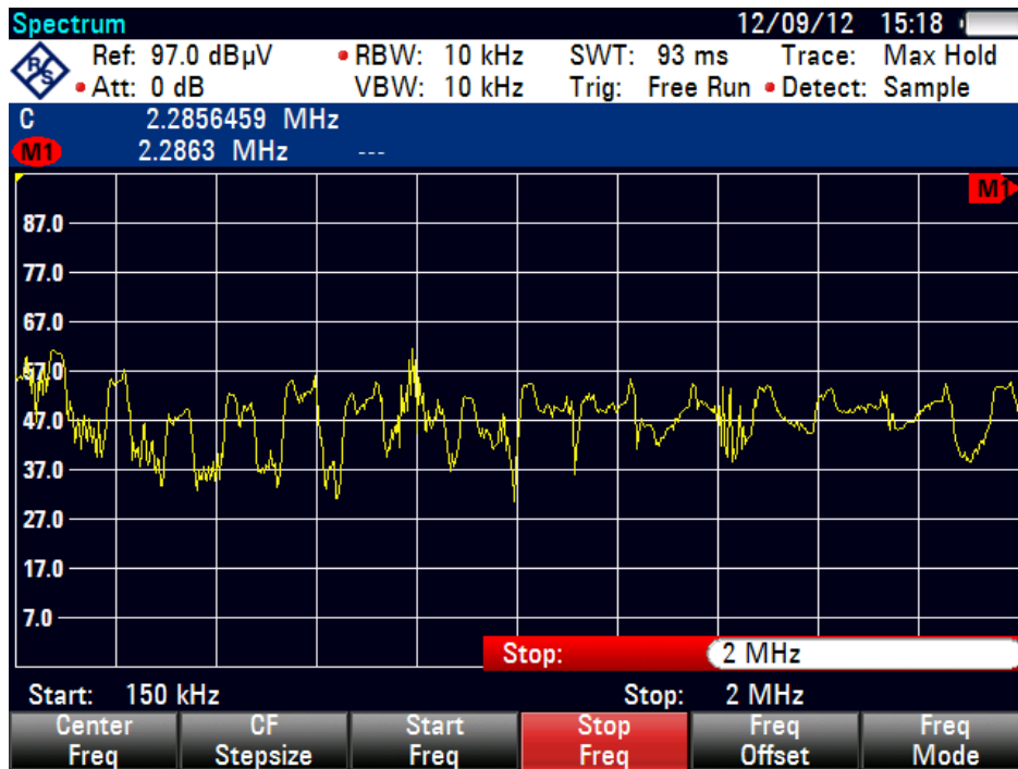
Figure 22. Conducted EMI Pre-compliance 150 kHz–2 MHz
