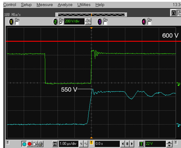
Figure 10. Maximum Output Power, V_{in} = 265 \text{ Vac} Note the good margin on the drain thanks to the low leakage term
