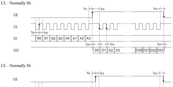
(Note) DO pin is an Nch open drain pin, so that the data varying time (tDC and tDH) differs depending on the pull-up resistance and substrate capacity.
