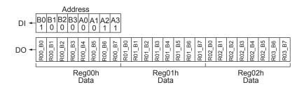
"C1" is input from LSB to the start as an address when the serial data is output from LV23401V, the controlled device is specified, and the mode as the data output is fixed. The subsequent data is output from DO pin synchronizing with lock (CL) after the address is input LSB from one with small register number. The output of data is ended by setting CE pin to Low.
