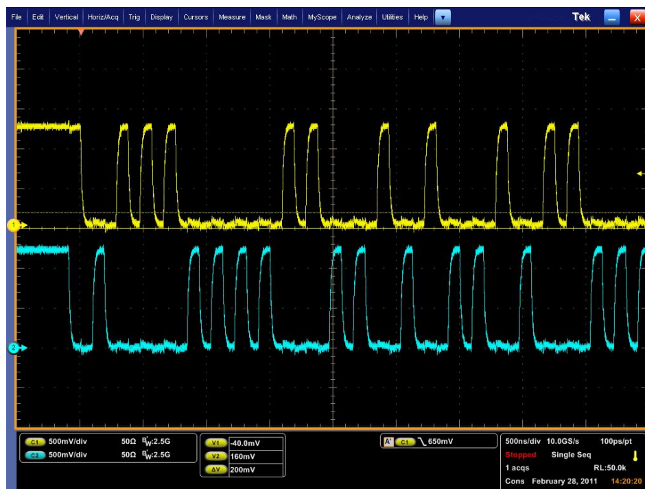
Figure 5. EMI4172 MIPI D-PHY LP Mode Measured Results
