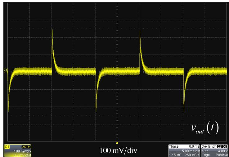
$V_{in} = 36 \text{ V} - 5 \text{ to } 10 \text{ A} - 1 \text{ A}/\mu\text{s}$
