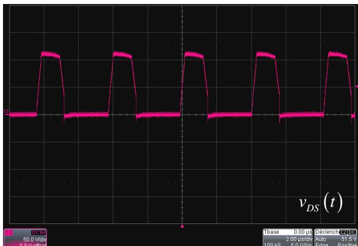
$$V_{in} = 36 \text{ V} - I_{out} = 0 \text{ A}$$
