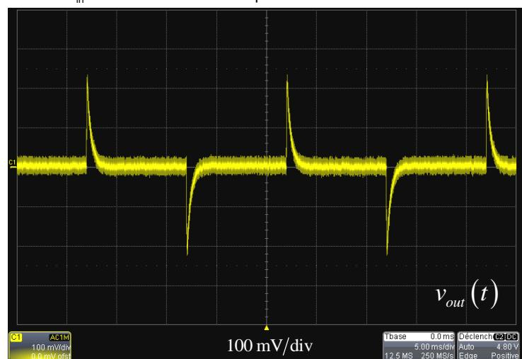
$V_{in} = 48 \text{ V} - 5 \text{ to } 10 \text{ A} - 1 \text{ A}/\mu\text{s}$
