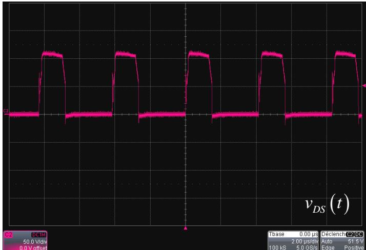
$$V_{in} = 36 \text{ V} - I_{out} = 10 \text{ A}$$
