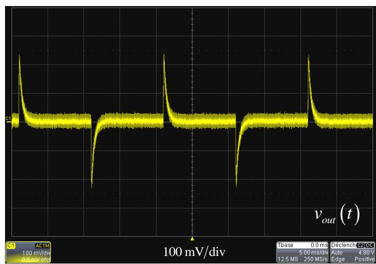
$V_{in} = 72 \text{ V} - 5 \text{ to } 10 \text{ A} - 1 \text{ A}/\mu\text{s}$
