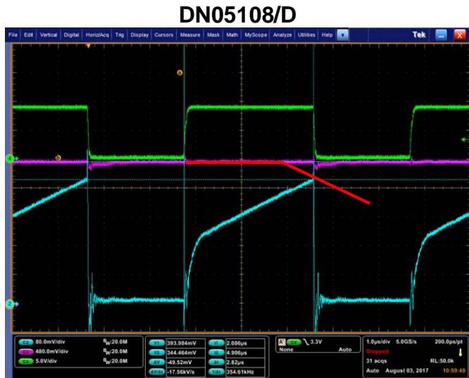
Figure 8: Slope Compensation Waveforms
