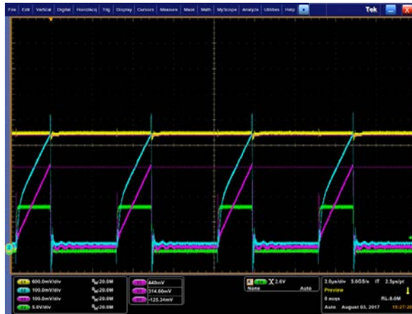
Figure 5: Over Power Protection Waveform
