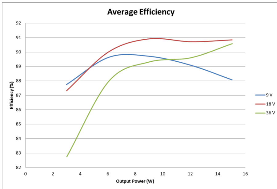
Figure 2: Average Efficiency vs Output Power
