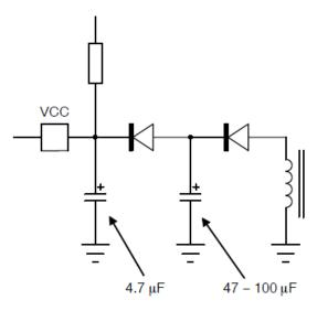
The 47uF capacitor does not load the Vcc terminal during start up thus assuring a fast start. After the converter starts switching, the 47uF capacitor provides a large energy storage element to keep the Vcc in the active region for a minimum of 50ms (the brown out detect period).
