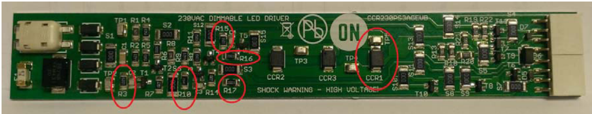
Figure 11. CCR230PS3AGEVB Evaluation Board with Changes Marked for DN05051/D
