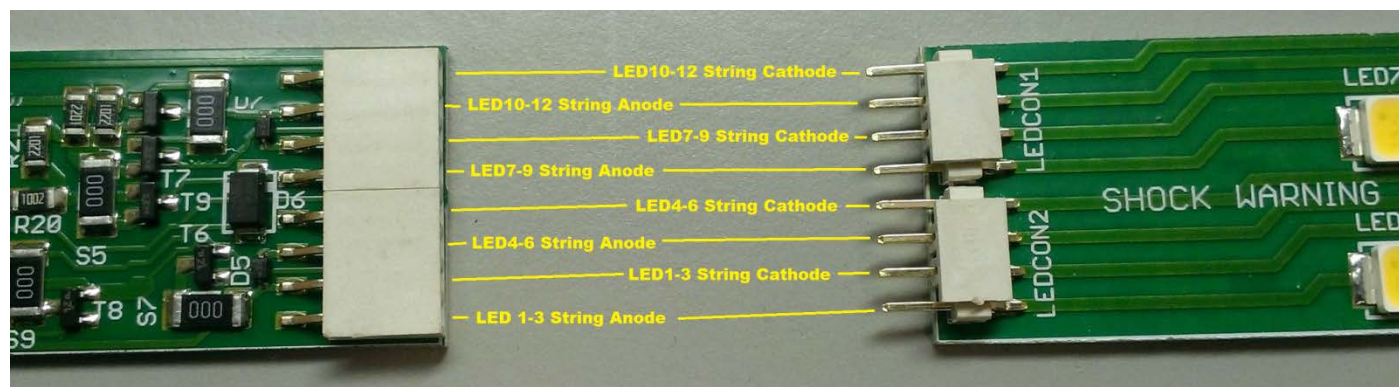
Figure 11: Connections to map to off-board LEDs. The circuit will not function in all three stages if one or more strings are connected incorrectly or missing.
