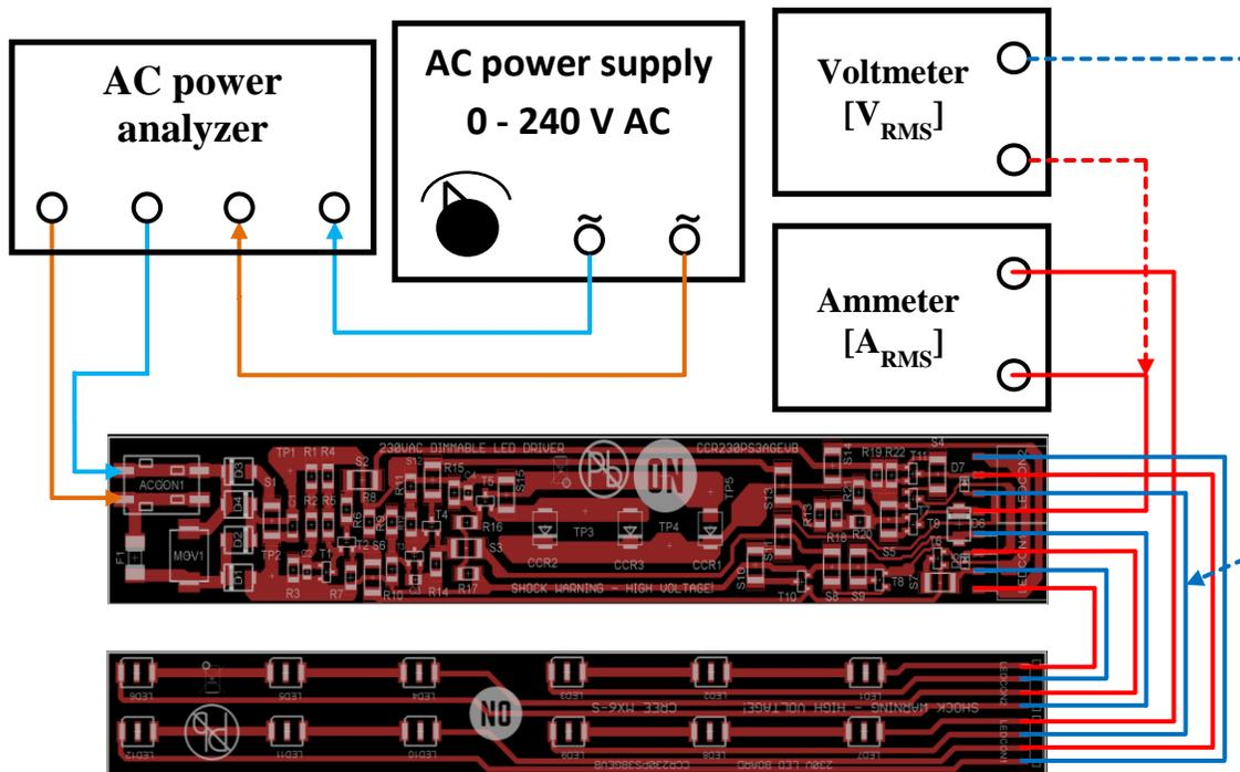
16. Turn AC power supply ON again. Allow circuit to run for 1 minute to stabilize for thermal settling before taking measurements.
