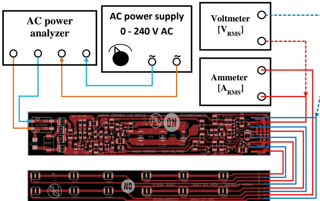
21. Turn AC power supply ON again. Allow circuit to run for 1 minute to stabilize for thermal settling before taking measurements.
