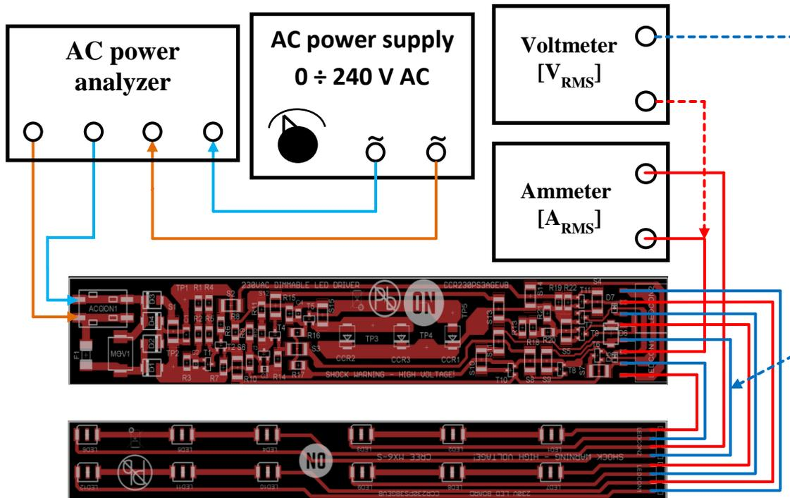
11. Turn AC power supply ON again. Allow circuit to run for 1 minute to stabilize for thermal settling before taking measurements.
