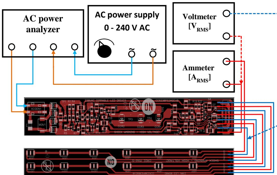
6. Turn AC power supply ON again. Allow circuit to run for 1 minute to stabilize for thermal settling before taking measurements.
