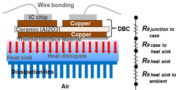
**Figure 13. Thermal Model of Power Module & Heatsink**
