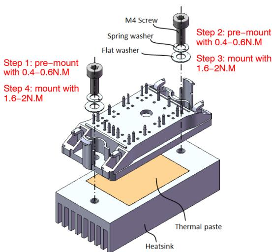
**Figure 33. Q0/Q1 Modules – Mounting to Heatsink**
