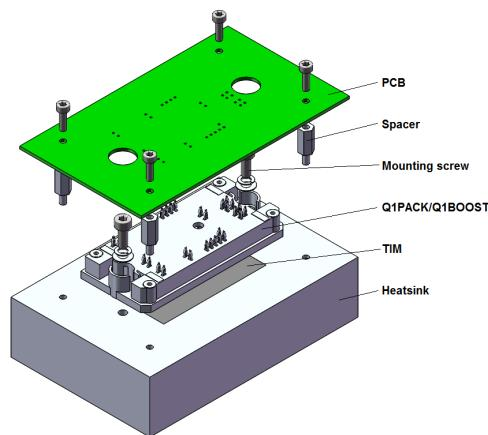
Figure 1. Q1 Module with PCB and Heatsink
