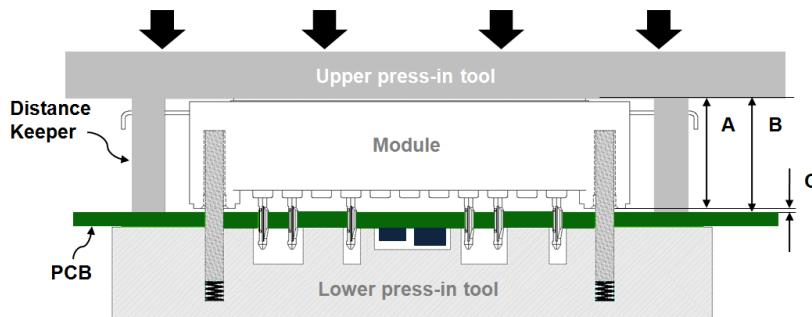
A: Package height (DBC bottom to case top) is  $12.00 \pm 0.30$  (mm)
