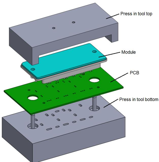
**Figure 19. Recommended Tooling Construction for the Press-in Process**
