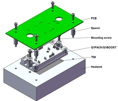
Figure 1. Q1 Module with PCB and Heatsink
