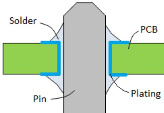
**Figure 29. Solder Wetting of PCB Through Hole**
