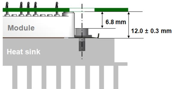
**Figure 38. Distance between PCB and Screw**
