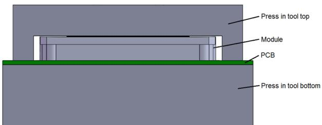
**Figure 20. Press-in Tools Closed, Module is Pressed in**
