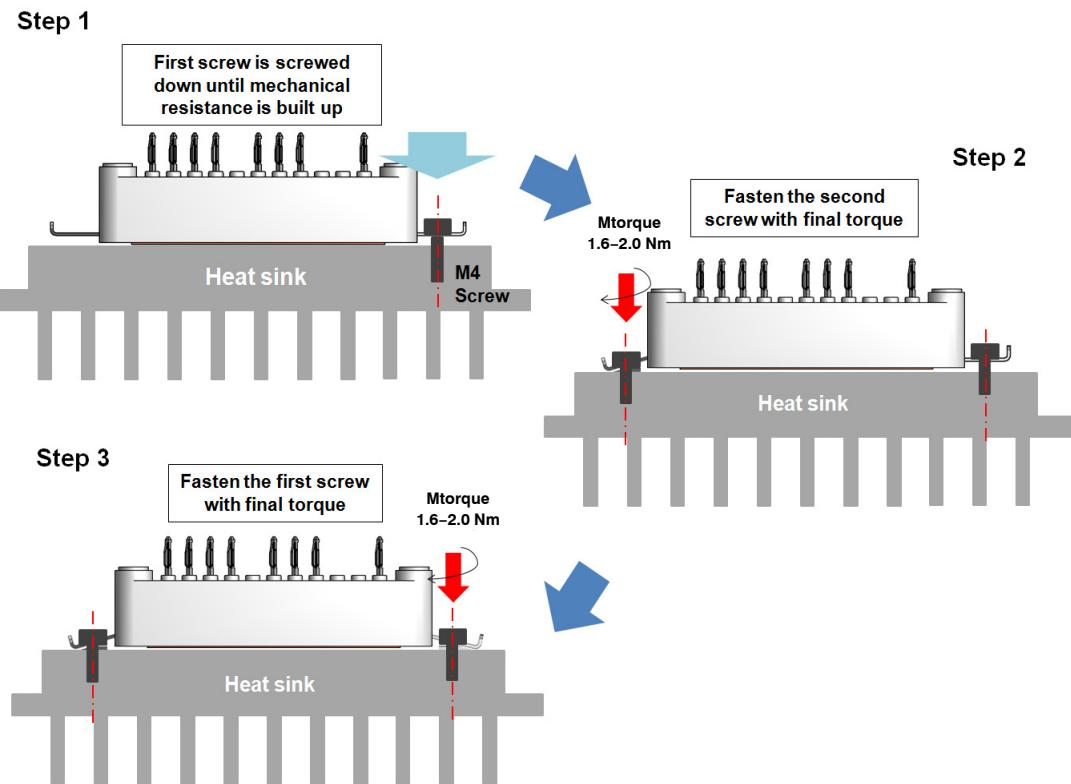
**Figure 32. Screw Clamping Steps (Method 2)**
