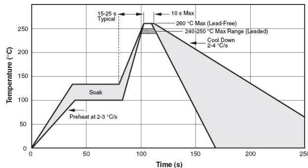
**Figure 30. Wave Solder Profile**
