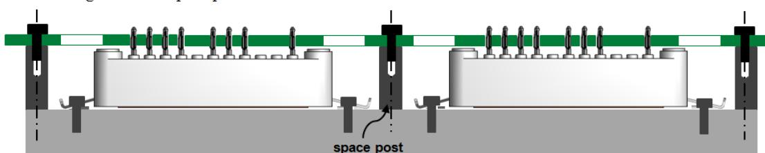
**Figure 37. Example of Whole Assembly Process for PCB and Heatsink with Space Posts**
