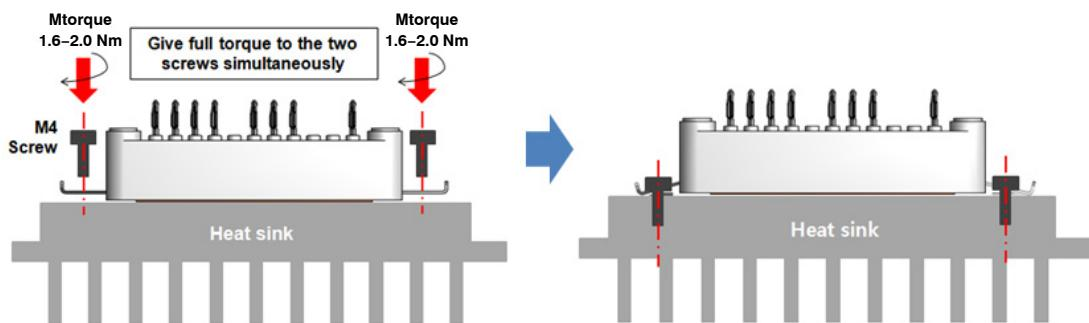
**Figure 31. Illustration of Screw Clamping with Heatsink (Method 1)**
