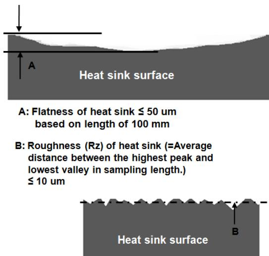
**Figure 14. Microscopic View of Surfaces.**
