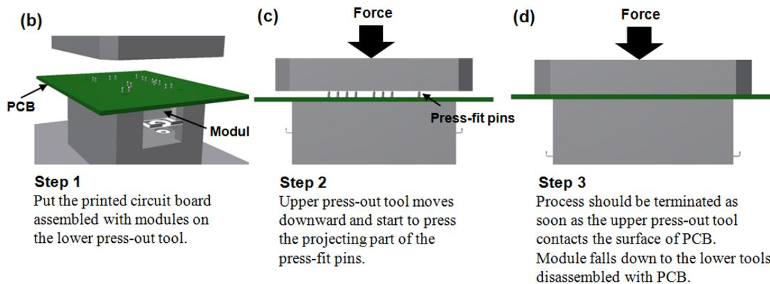
Figure 27. Press-out Process
