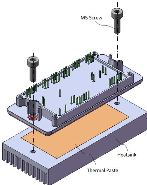
Figure 34. Q2 Modules – Mounting to Heatsink
