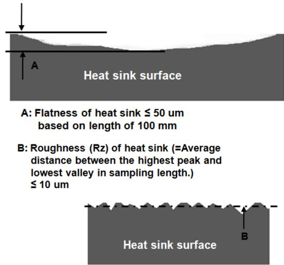
**A: Flatness of heat sink  $\leq 50 \mu m$  based on length of  $100 mm$**
