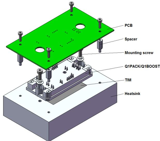
**Figure 12. Q1 Package Mounting Example**
