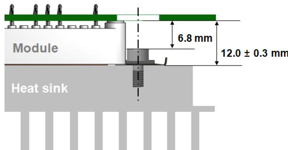
Figure 38. Distance between PCB and Screw
