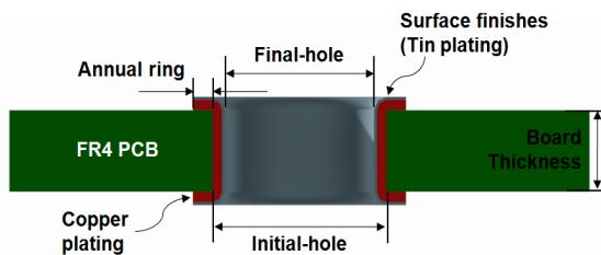
**Figure 3. Cross-section of PCB**
