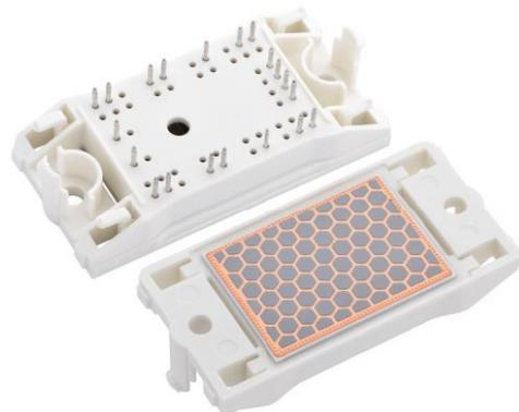
**Figure 17. Printing Pattern Example for TIM Material**
