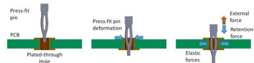
Figure 2. Press-fit Process
