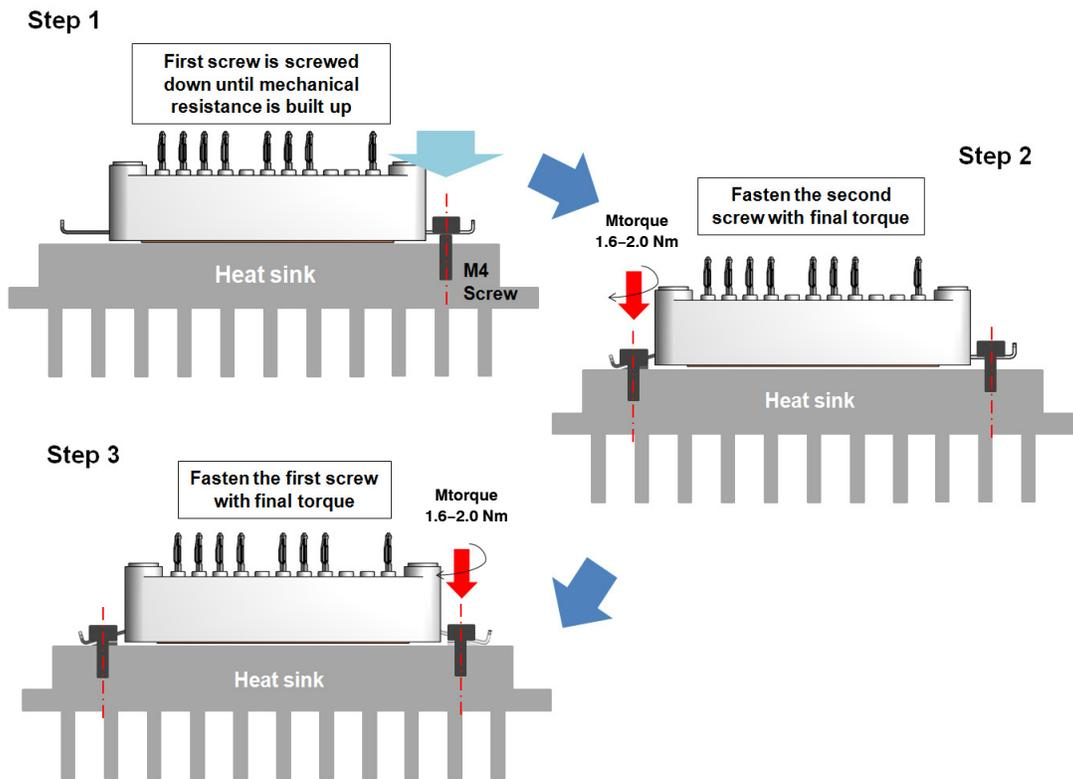
**Figure 32. Screw Clamping Steps (Method 2)**
