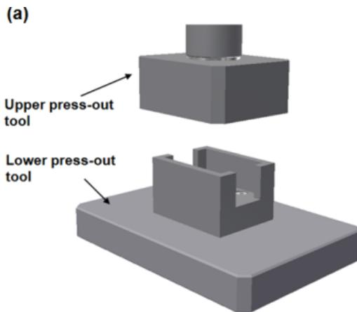
Press-out tool consists of two parts; upper press-out tool and lower press-out tool should be aligned in parallel with each other.
