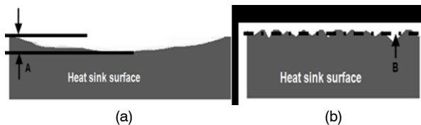
Figure 17. Flatness (a) and Roughness (b) of the Heatsink
