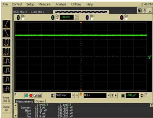
Figure 5. SiPM signal when exposed to full ambient light (100 mV, 5 ms)
