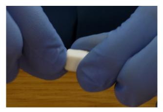
Figure 7. Pinch Together the Overlapping Ends of the Teflon Tape to Seal the Face Opposite the Exit Surface of the Crystal. Ensure that it is Done Tightly so that it Remains Secure
