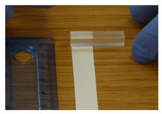
Figure 1. Ensure that the Crystal is Clean and Free of Marks from Finger-prints etc. Carefully Lay the Crystal onto the Tape, Ensuring that the Exit Face Edge is Aligned to the Edge of the Tape
