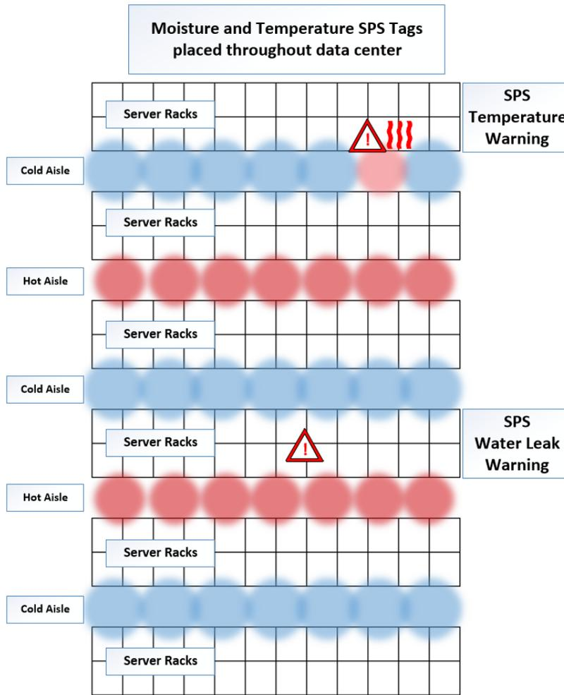
Figure 3. Data Center-wide SPS Solution
