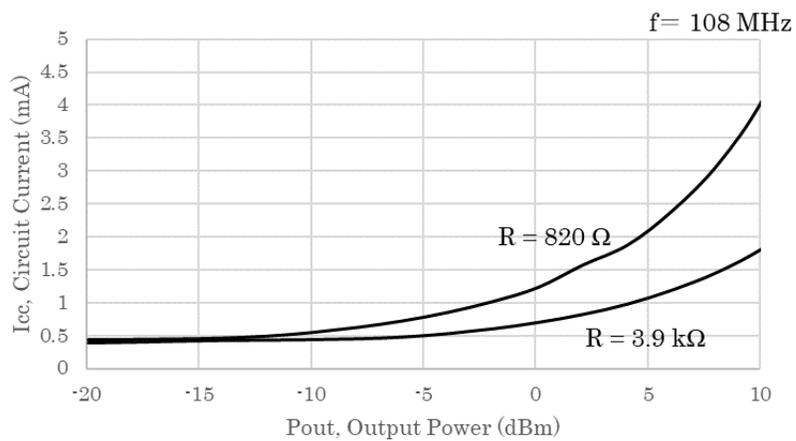
Figure 12. Pin - I<sub>cc</sub> (f = 108 MHz)
