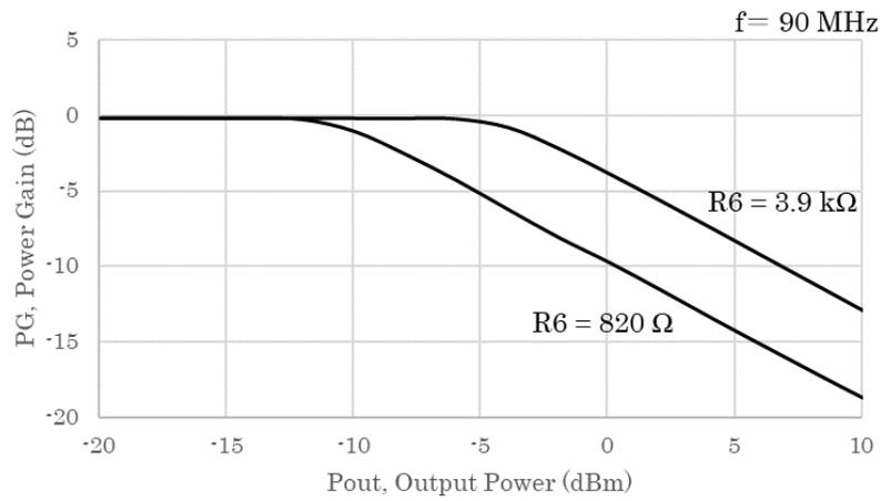
Figure 8. Pin - PG (f = 90 MHz)
