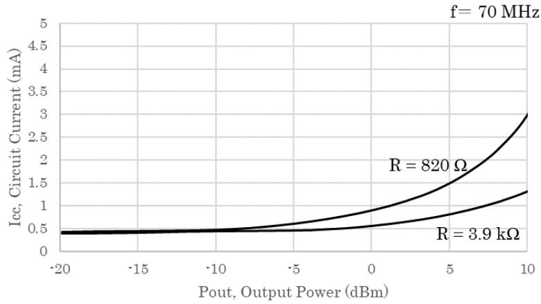
Figure 10. Pin - I<sub>cc</sub> (f = 70 MHz)
