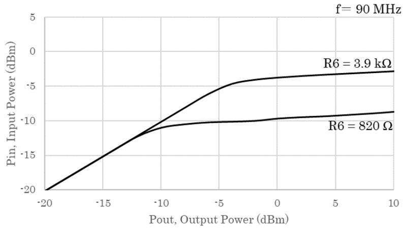
Figure 5. Pin – Pout (f = 90 MHz)
