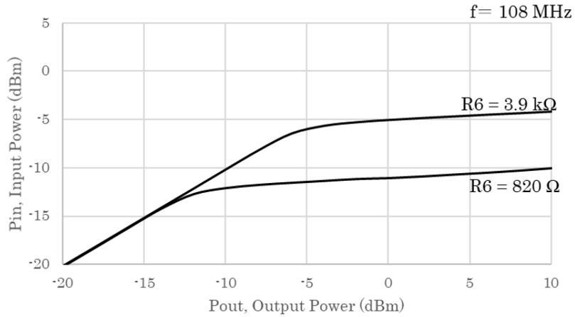
Figure 6. Pin – Pout (f = 108 MHz)
