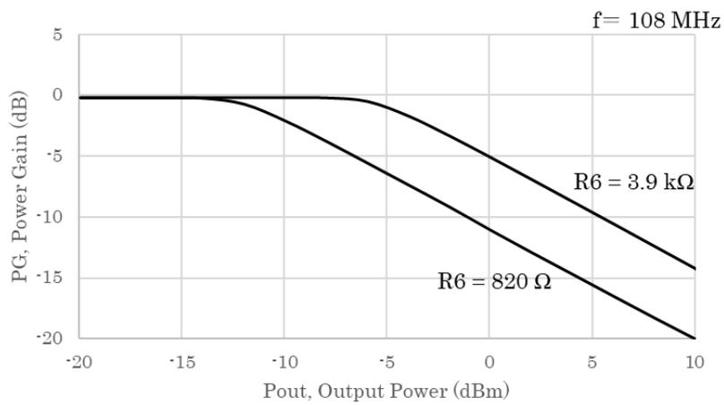
Figure 9. Pin - PG (f = 108 MHz)
