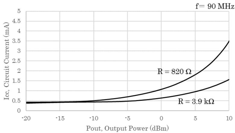
Figure 11. Pin - I<sub>cc</sub> (f = 90 MHz)
