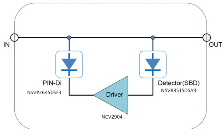
**Figure 2. Block Diagram**
