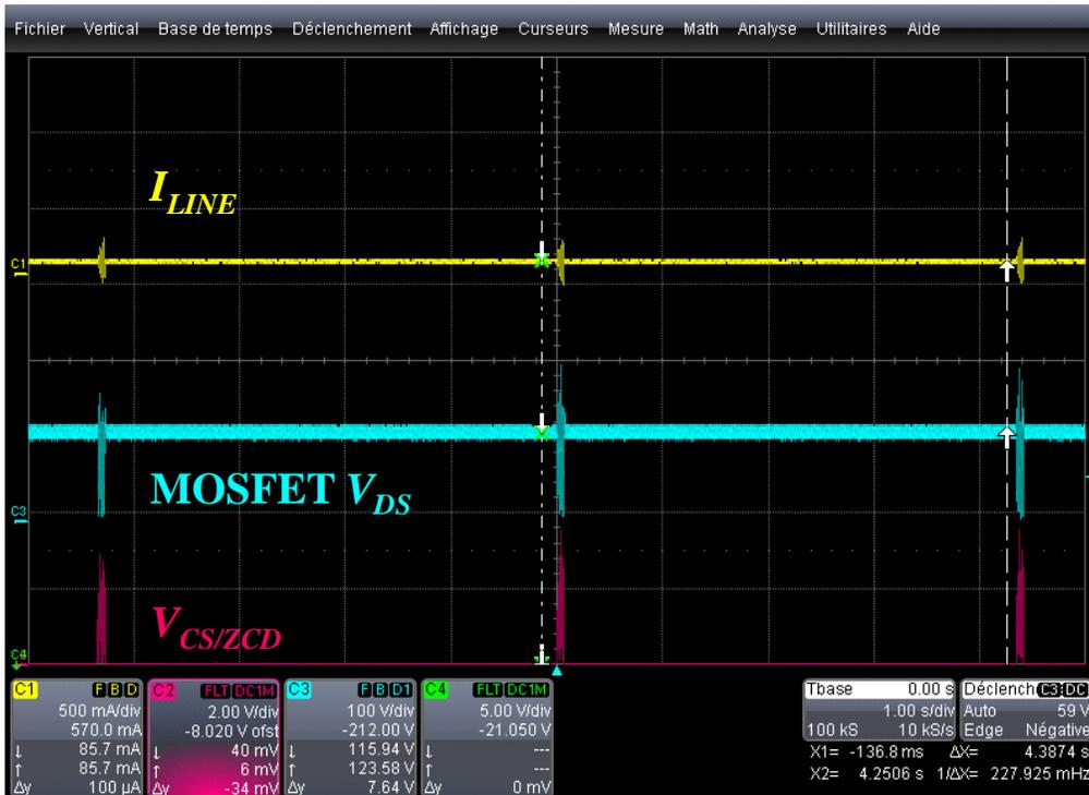
Figure 15. Auto-recovery Mode in Over-voltage Condition (Open LED String)
