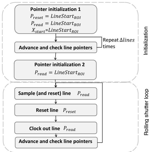
Note that two lines are reset during a step of the rolling shutter loop: First the P.read line is reset to provide the R-value for the readout. Secondly, the line P.reset is reset in order to control the integration time.
