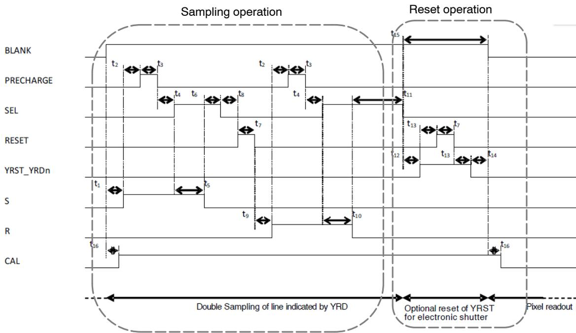
Note that the "Sampling operation" indicated above resets the photodiode after the S-value has been sampled, so that an R value may be provided for uncorrelated double sampling. Hence, each line operation contains two resets: One for the photodiode being read out, and a second for the photodiode on the reset-line.
