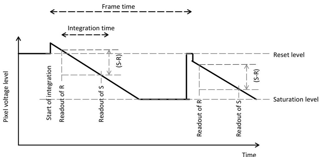
Figure 1. Principle of Correlated Double Sampling Eliminating kTC-noise
