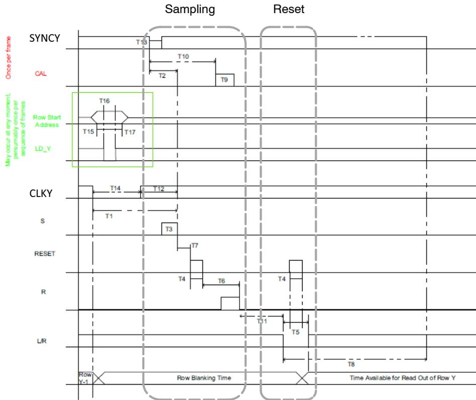
Note that the "Sampling operation" indicated above resets the photodiode after the S-value has been sampled, so that and R value may be provided for uncorrelated double sampling. Hence, each line operation contains two resets: One for the photodiode being read out, and a second for the photodiode on the reset-row.
