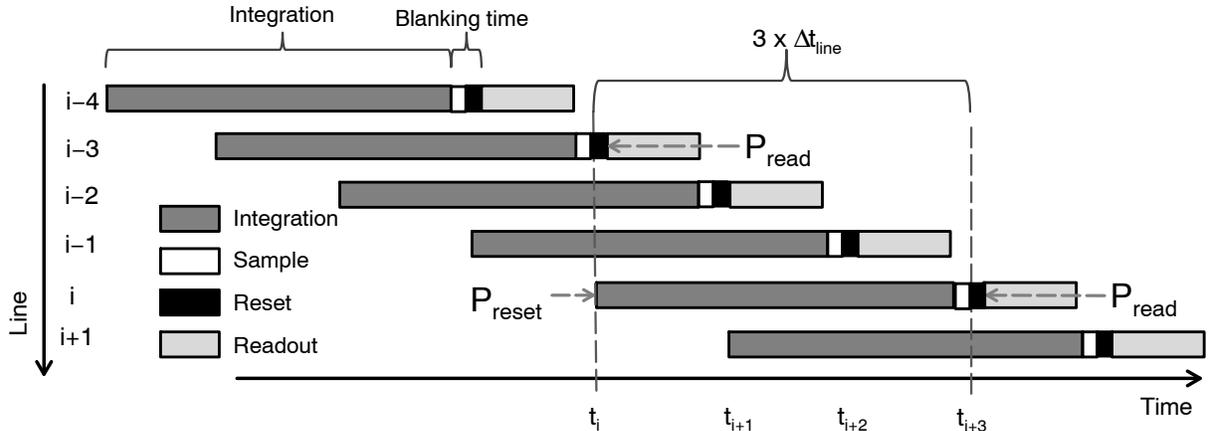
**Figure 4. Rolling Shutter Operations Illustrated in Line-per-line Form**
