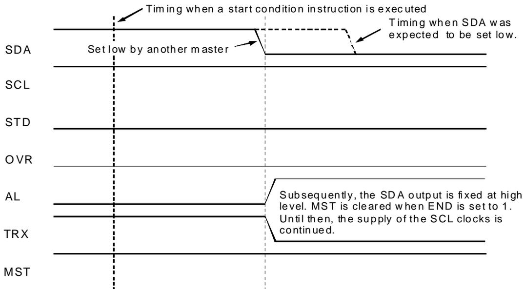
**Figure 3.30.10 Arbitration Lost During Start Condition Generation <2>**
