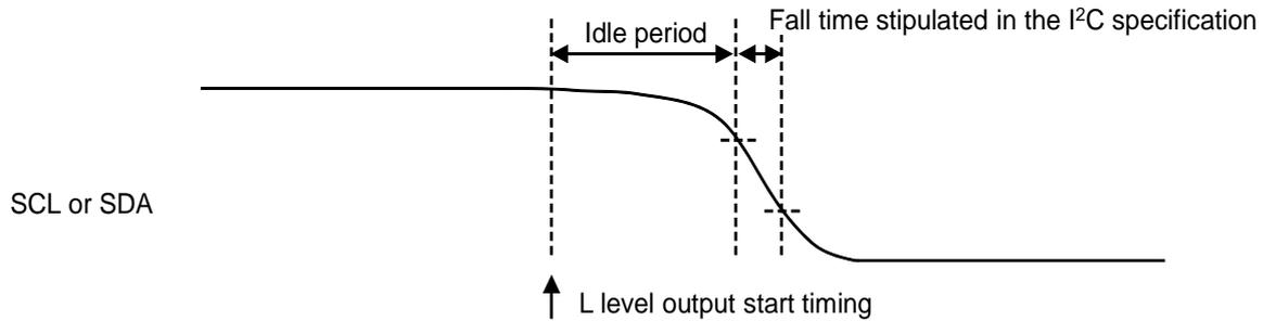
Figure 3.29.2 I<sup>2</sup>C Port Falling Waveform
