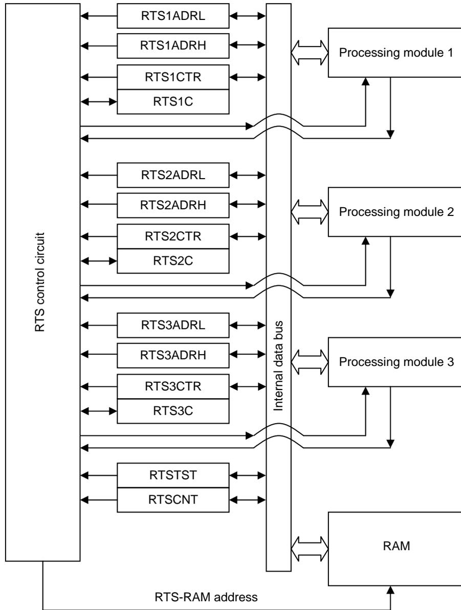
Figure 3.34.1 RTS Block Diagram
