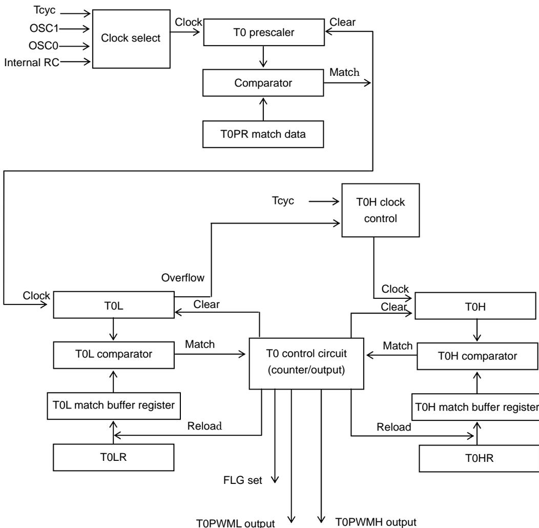
Figure 3.16.1 Timer 0 Block Diagram
