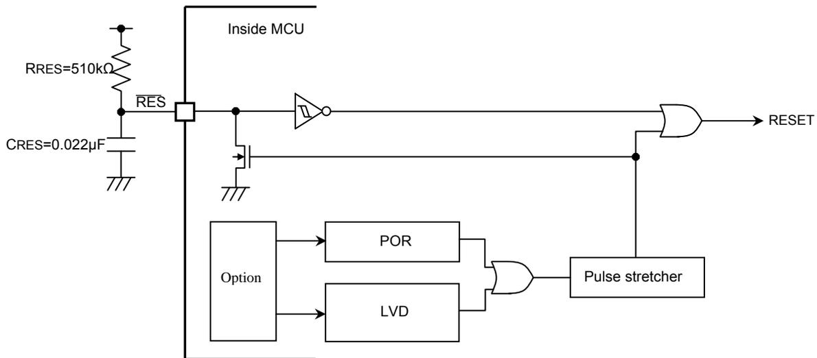
Figure 4-6-1 : Internal Reset Circuit configuration diagram
