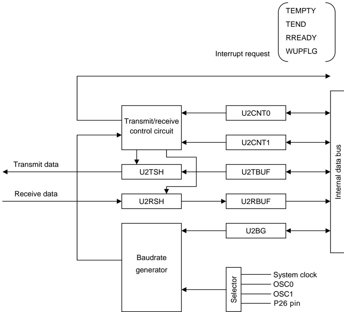
Figure 3.24.1 UART2 Block Diagram
