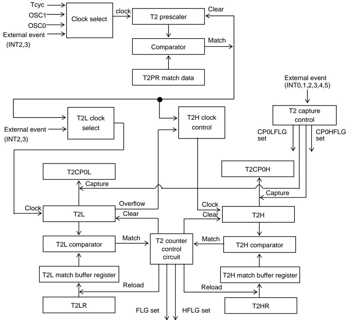
Figure 3.18.2 Timer 2 Block Diagram
