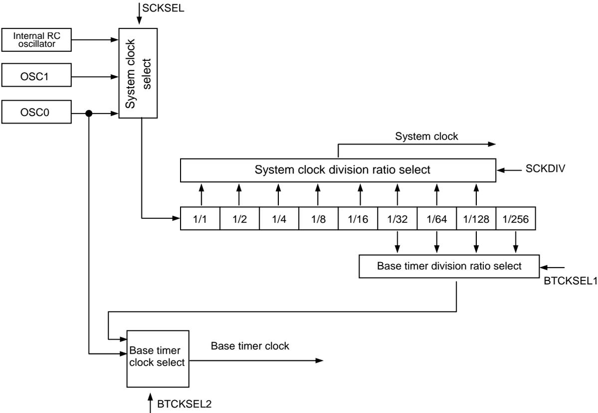
**Figure 4.2.1 System Clock Generator Circuit Block Diagram**
