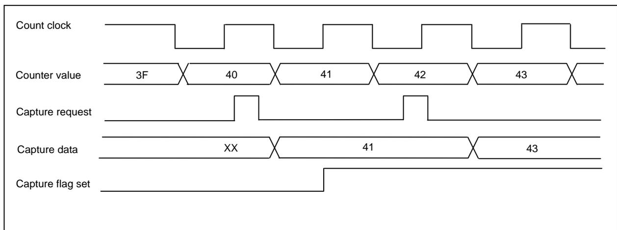
Figure 3.18.1 Capture Timing
