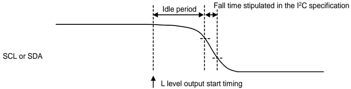
Figure 3.30.2 I<sup>2</sup>C Port Falling Waveform
