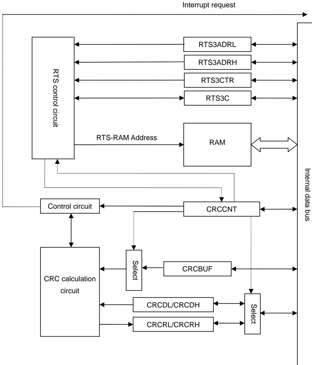
**Figure 3.35.1 RTS Block Diagram**
