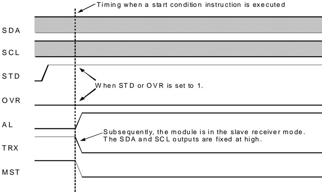
**Figure 3.30.9 Arbitration Lost During Start Condition Generation <1>**
