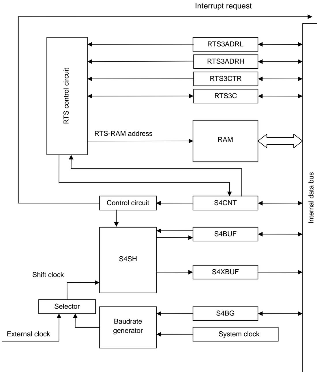
Figure 3.28.1 SIO4 Block Diagram
