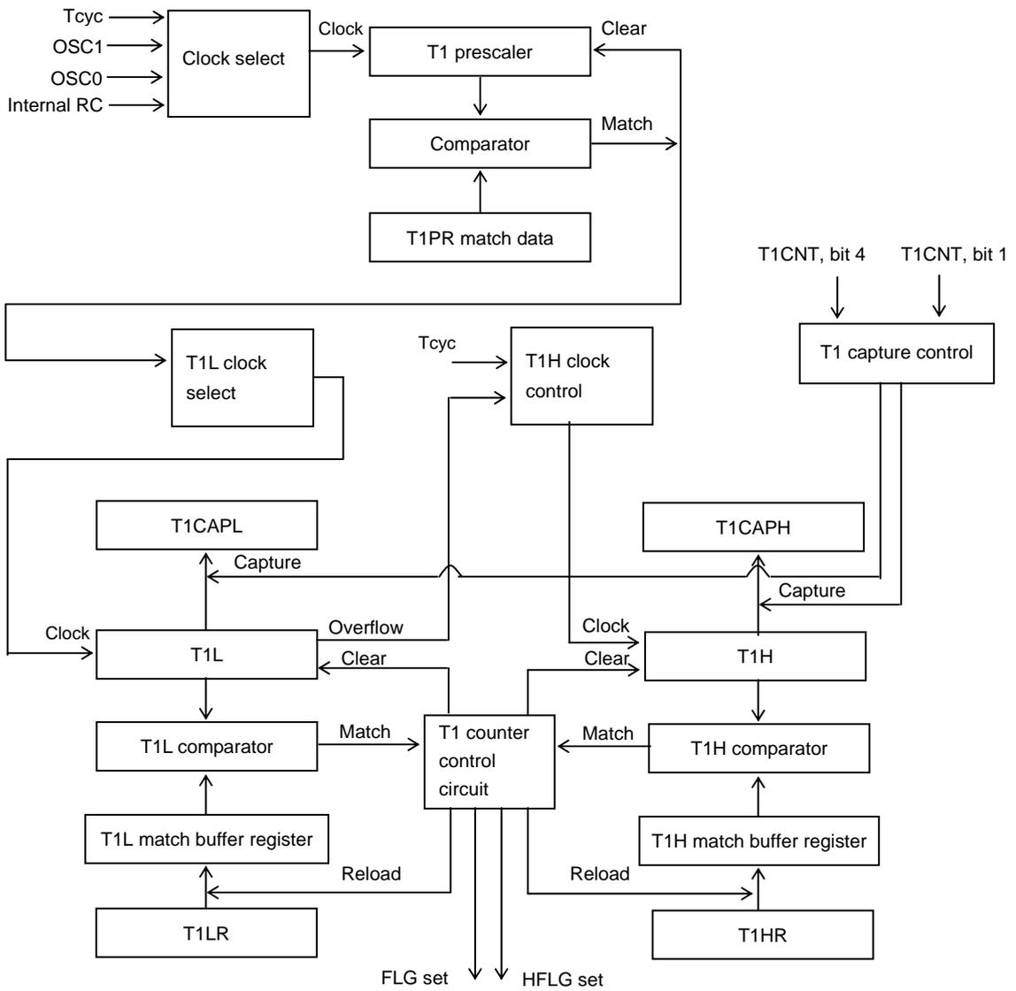
Figure 3.17.1 Timer 1 Block Diagram
