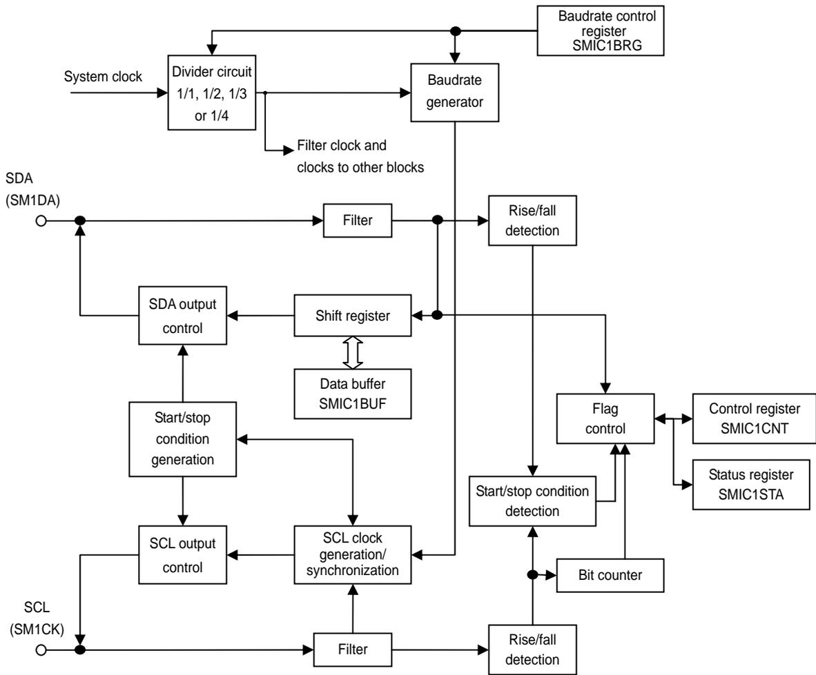
Figure 3.30.1 SMIC1 Block Diagram
