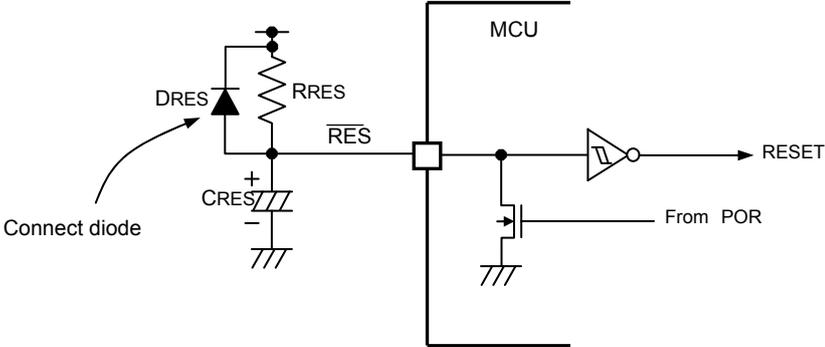
Figure 4-6-8 : External POR reset circuit configuration example
