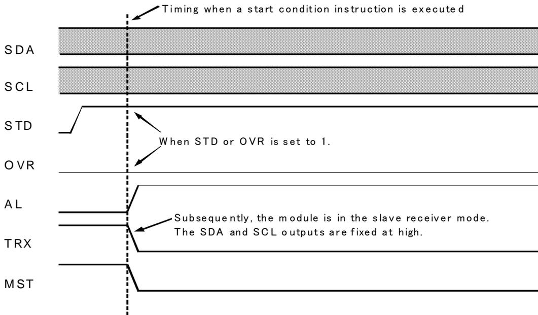
**Figure 3.29.9 Arbitration Lost During Start Condition Generation <1>**
