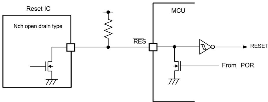
Figure 4-6-6 : Reset circuit configuration diagram In case of using Nch Open drain type
