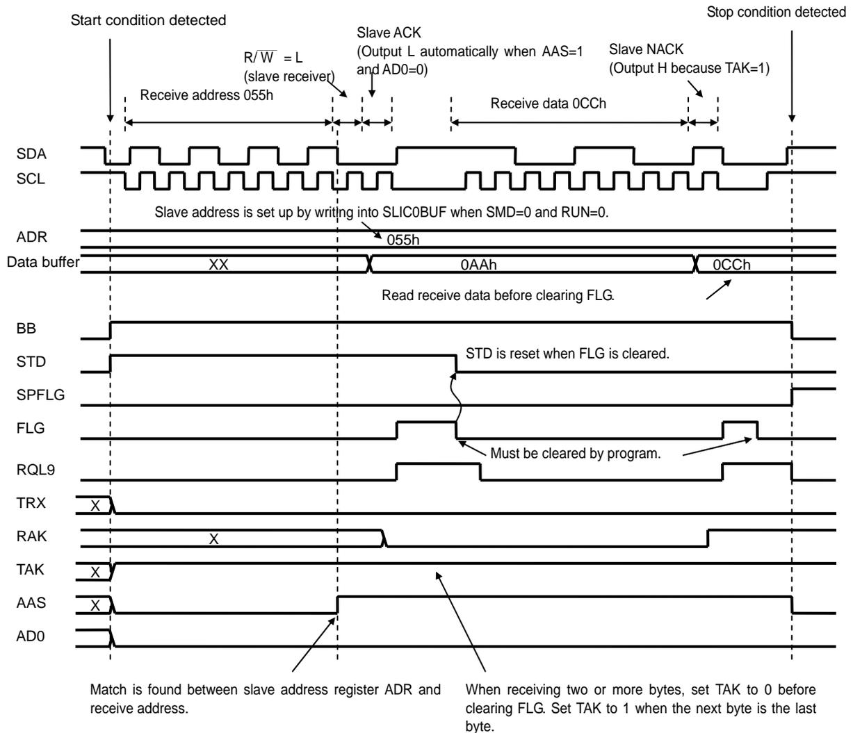
Figure 3.31.5 I<sup>2</sup>C Mode 1-byte Reception Timing Diagram
