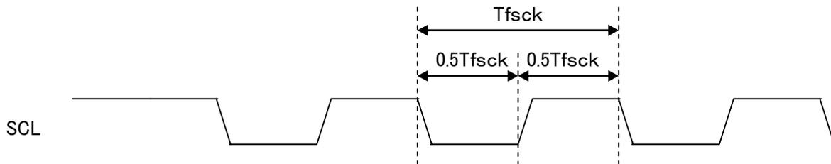
Figure 3.29.3 SCL Clock Waveform
