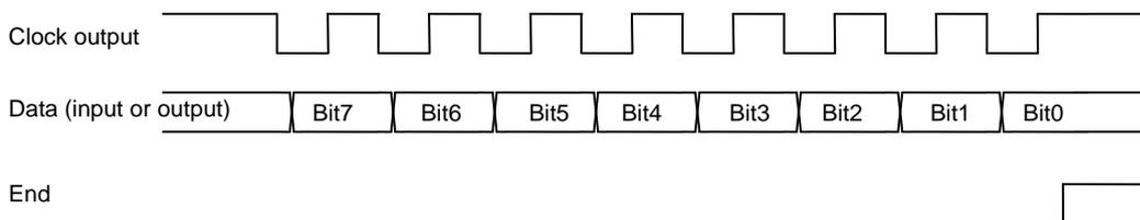
Figure 3.31.4 Waveform of Simple SIO Mode 1-byte Transmission/Reception
