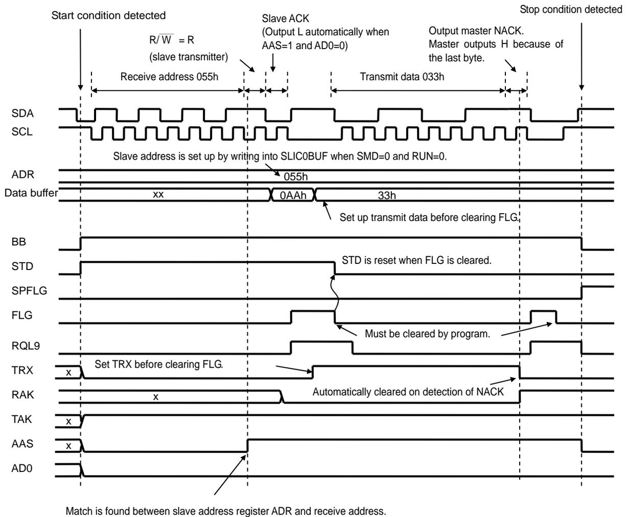
Figure 3.31.7 I<sup>2</sup>C Mode 1-byte Transmission Timing Diagram
