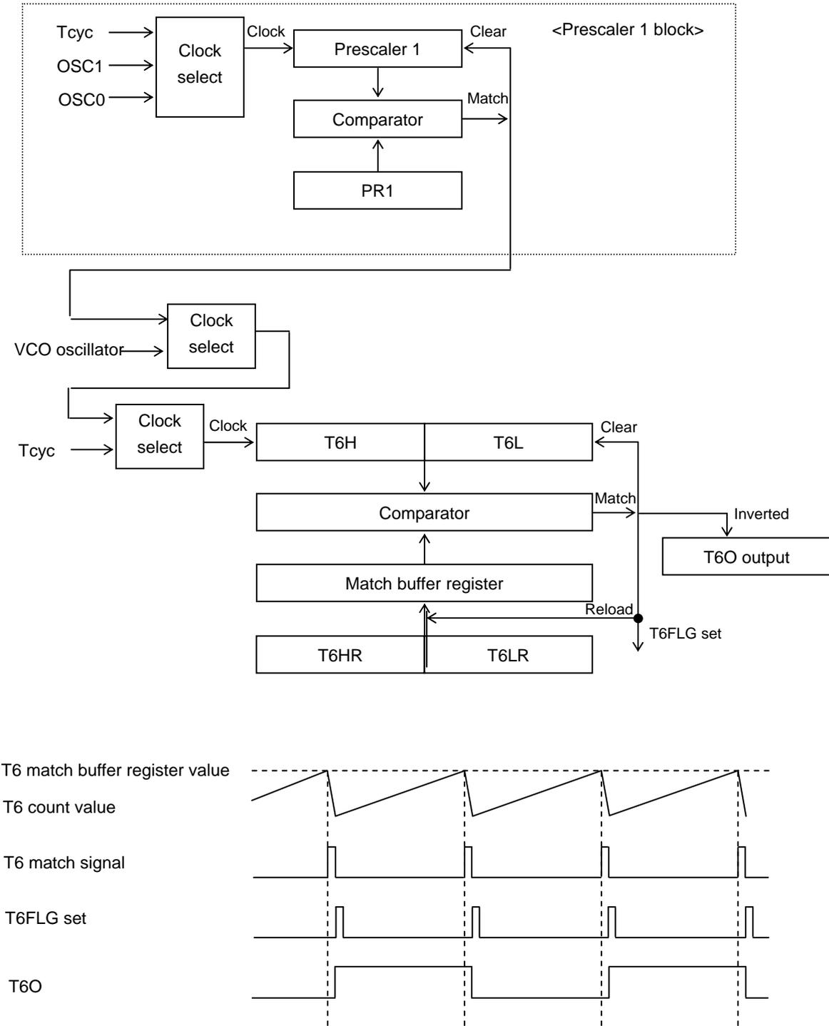
Figure 3.21.1 Timer 6 Block Diagram
