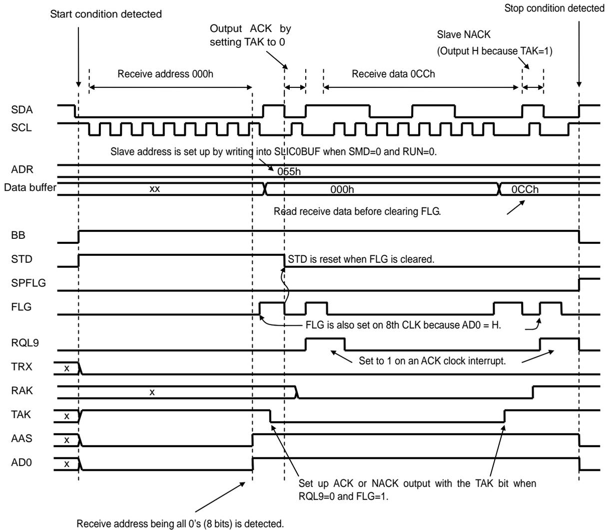
Figure 3.31.6 I<sup>2</sup>C Mode 1-byte Reception Timing Diagram (General Call)
