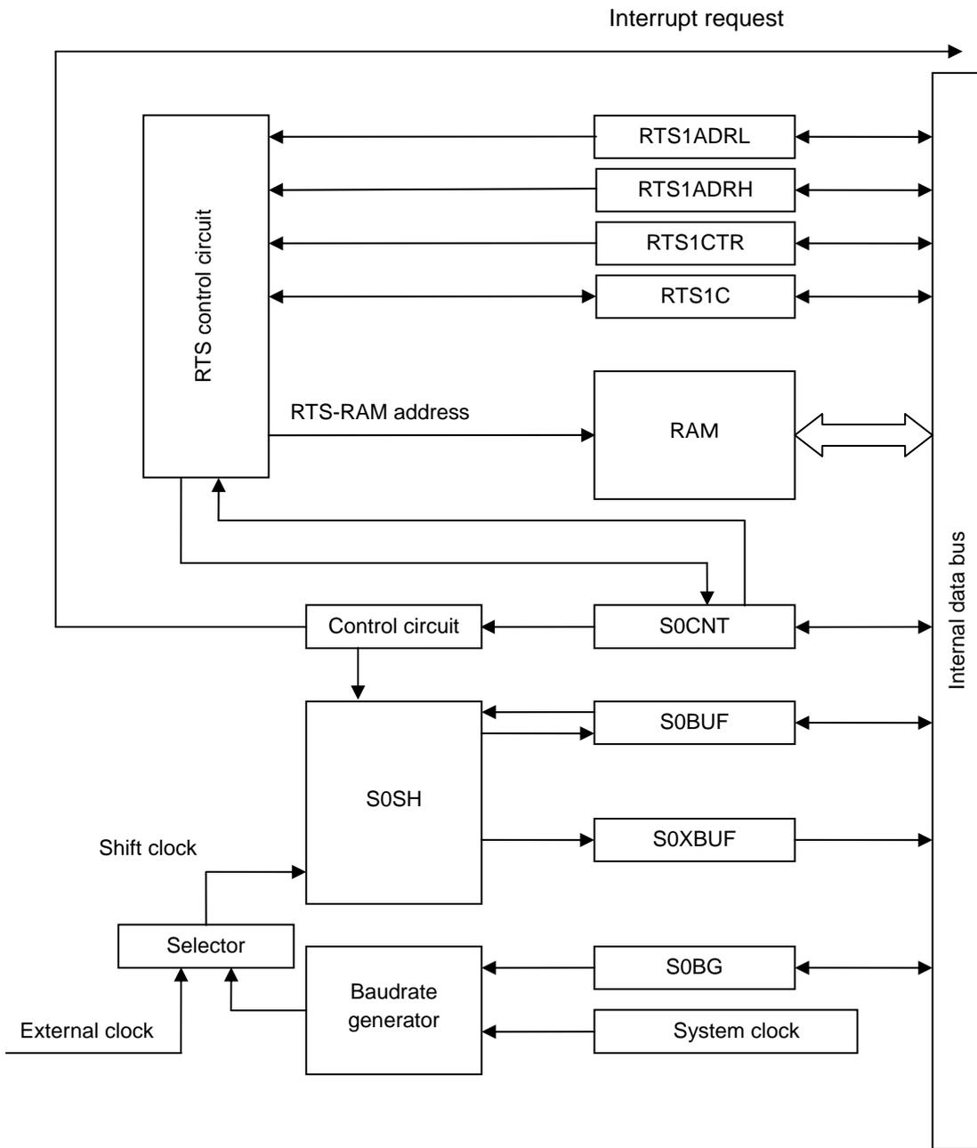
Figure 3.26.1 SIO0 Block Diagram
