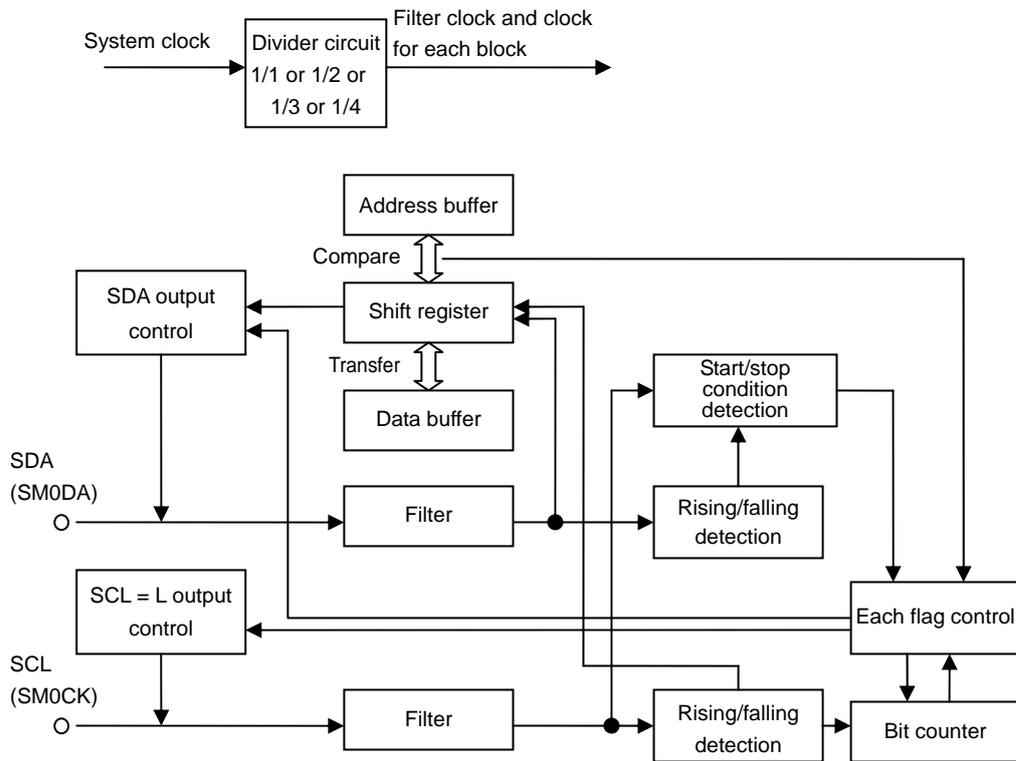
Figure 3.31.1 SLIC0 Block Diagram
