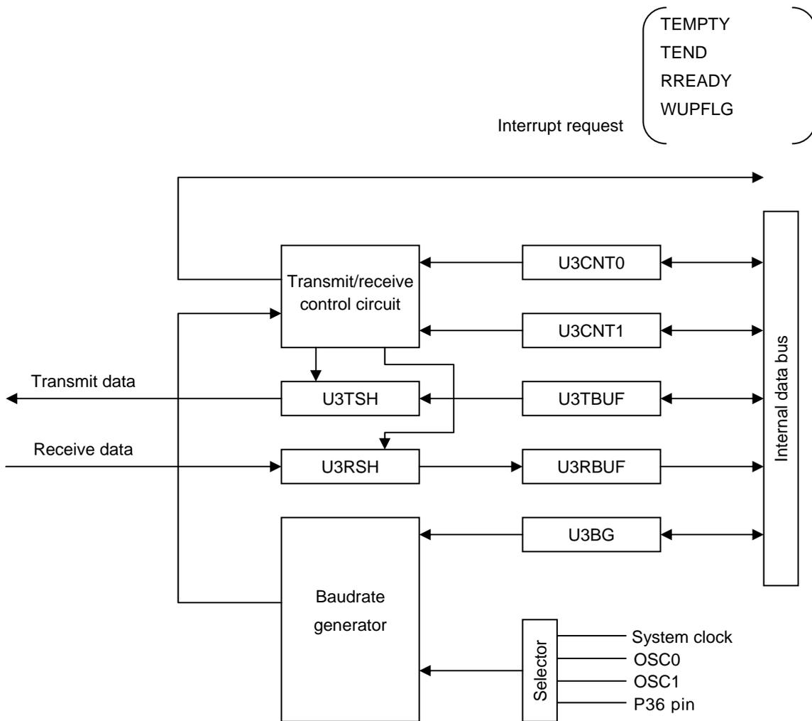
Figure 3.25.1 UART3 Block Diagram
