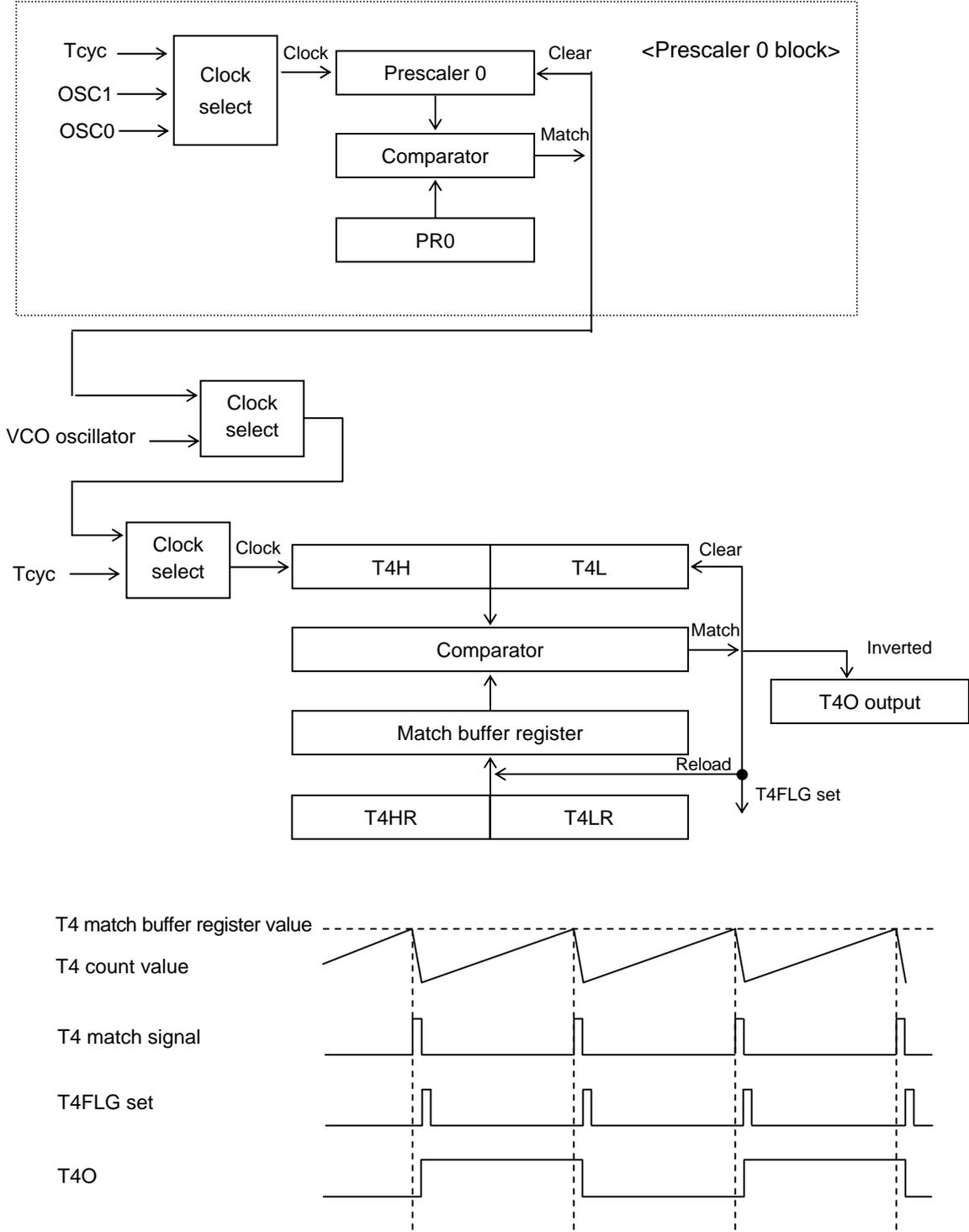
Figure 3.20.1 Timer 4 Block Diagram
