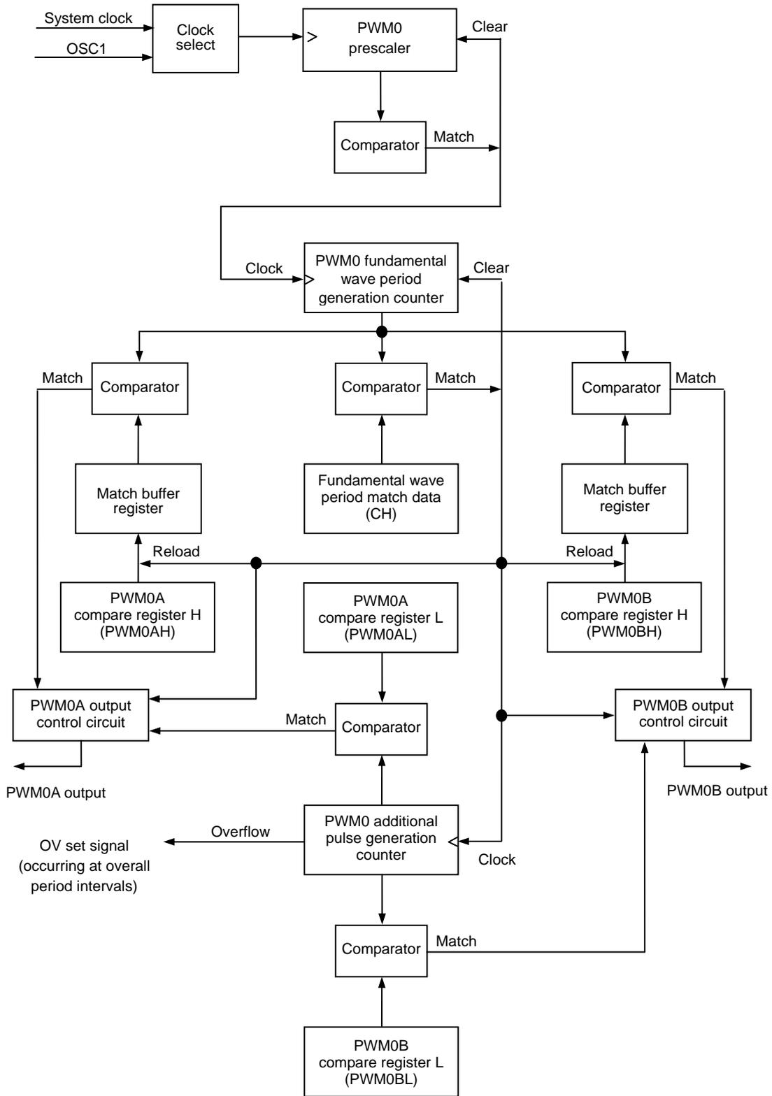
**Figure 3.32.1 PWM0 Block Diagram**
