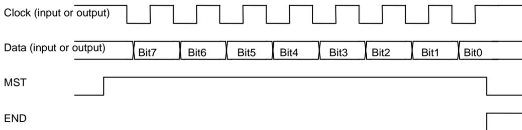
Figure 3.30.11 Waveforms of Simple SIO Mode 1-byte Transmission/Reception
