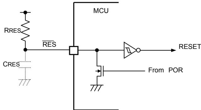
Figure 4-6-2 : Reset circuit configuration example
