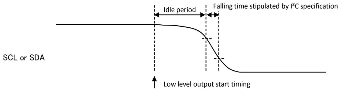
Figure 3.31.2 I<sup>2</sup>C Port Falling Edge Waveform
