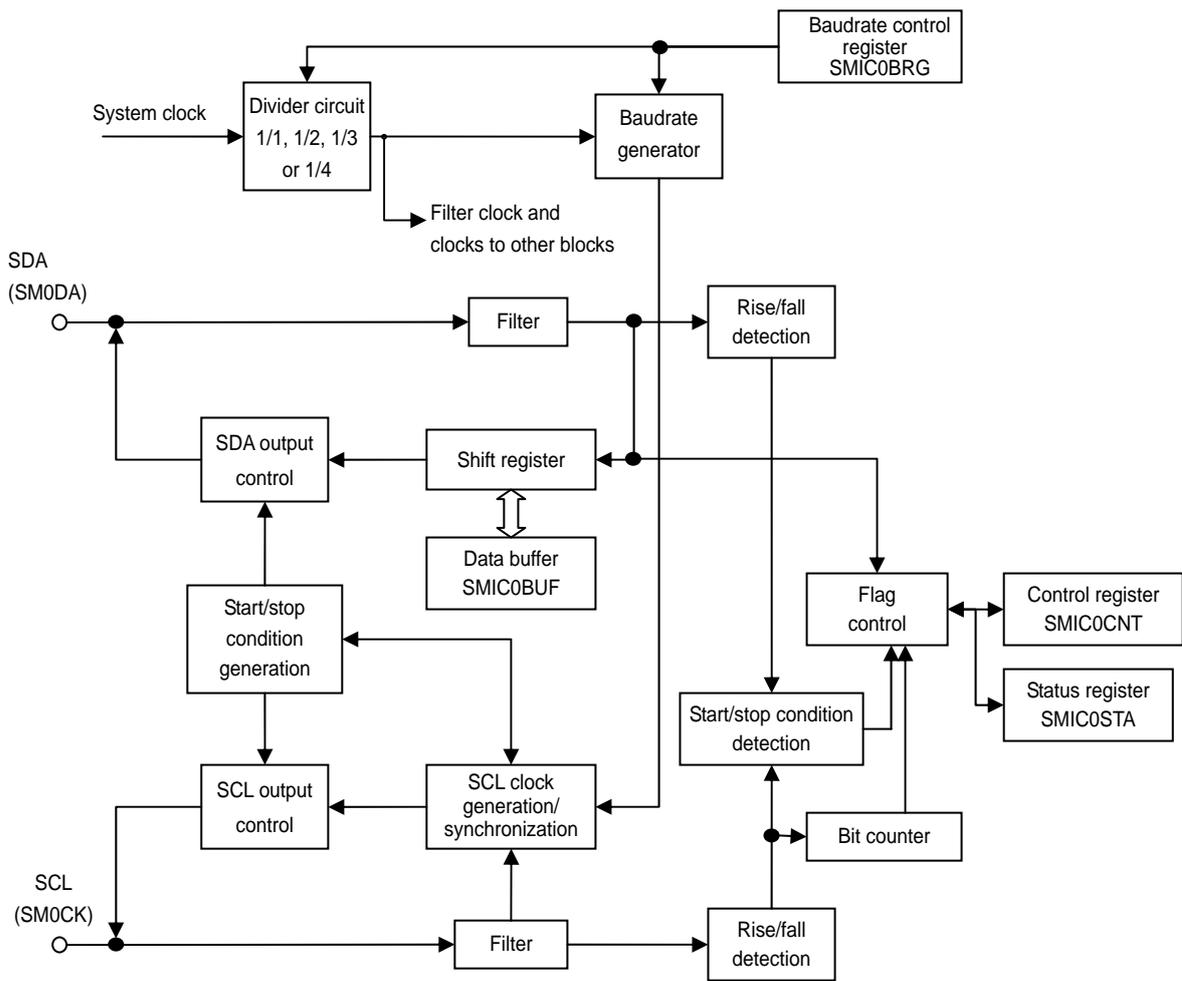
Figure 3.29.1 SMIC0 Block Diagram
