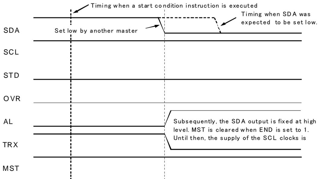
**Figure 3.29.10 Arbitration Lost During Start Condition Generation <2>**
