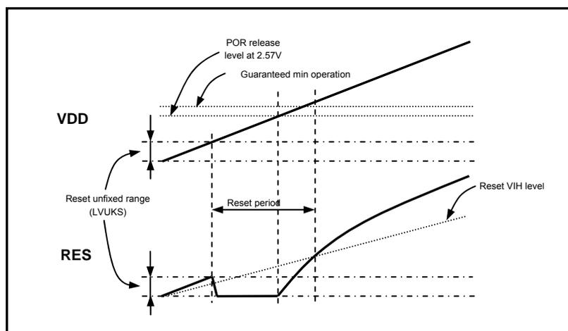
Figure 4-6-3 : Example of Release level waveform
