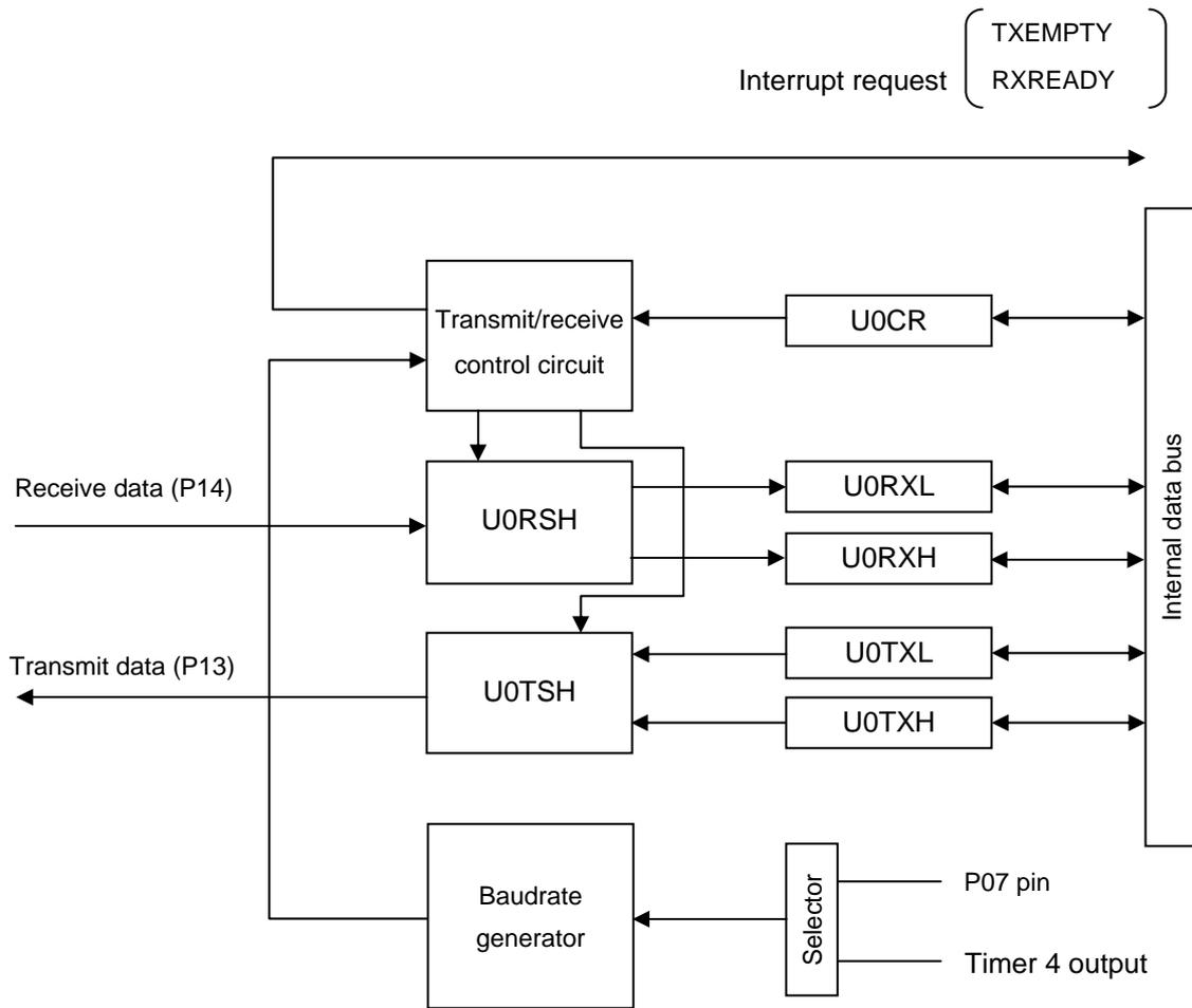
Figure 3.23.1 UART0 Block Diagram
