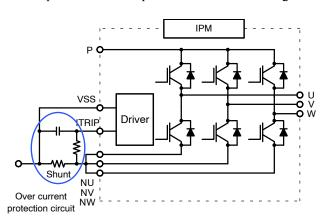
Figure 9. Over-Current Protection Circuit
