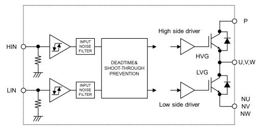
Figure 14. Cross-Conduction Prevention
