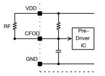
Figure 23. CFOD Circuit (STK5C4U332J-E)
