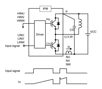
Figure 5. Switching Loss Measurement Circuit
