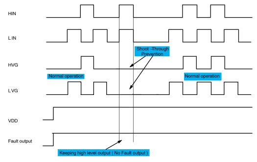
Figure 15. Cross-Conduction Prevention Timing Diagram
