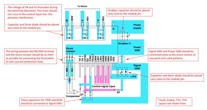
Figure 18. Compact IPM Recommended Layout
