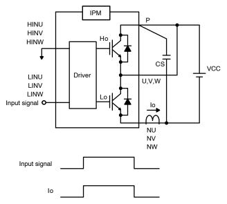
Figure 7. Short Circuit Operating Area Measurement Circuit
