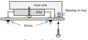
Figure 27. Fix to Heat Sink
