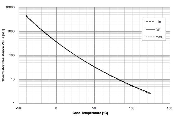
Figure 8. NTC Thermistor Resistance versus Temperature
