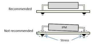
Figure 28. Mounting Position on PCB
