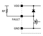
Figure 21. Fault Connection
