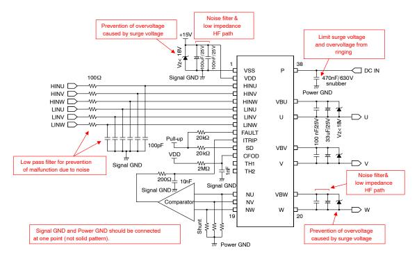
Figure 17. Compact IPM Series Application Circuit
