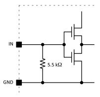
Figure 20. Internal Input Circuit
