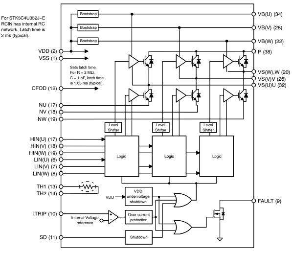
Figure 2. Compact IPM Series Internal Diagram
