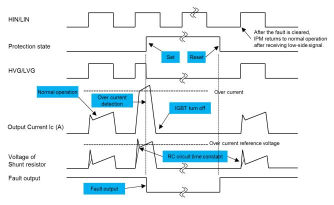
Figure 11. Overcurrent Protection Timing Diagram
