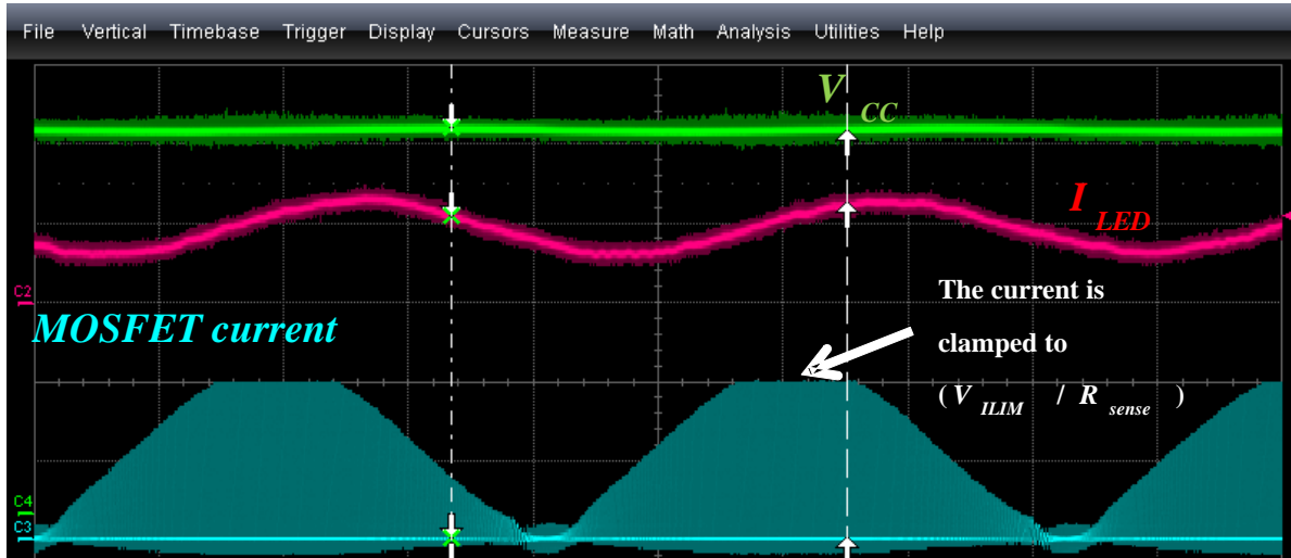
Figure 2. Current Over-Current Limitation ( V_{ILIM} is Over-Current Threshold, R_{SENSE} the Current Sense Resistor)
