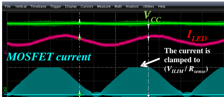
Figure 1. Current Over-current Limitation ( V_{ILIM} is the Over-current Threshold, R_{sense} the Current Sense Resistor)
