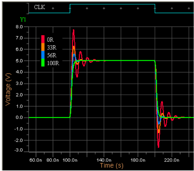
Figure 17. RxD Trace Impedance Mismatch Compensation (2-Layer PCB, ringing at MCU input pin)
