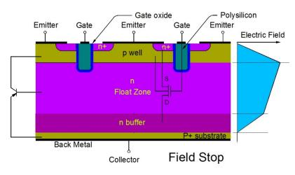
Figure 7. Field Stop IGBT Diagram
