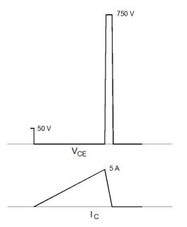
Figure 3. UIS Test Waveforms
