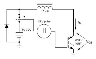
Figure 2. UIS Test Circuit
