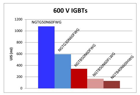
Figure 4. UIS Ratings for ON Semiconductor 600 Volt IGBTs
