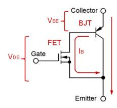
Figure 1. IGBT Current Flow
