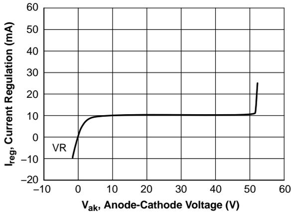
Figure 4. Typical I-V Characteristic of a CCR
