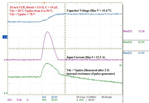
Figure 7. For Pulse 2a with 28  $V_{dc}$  + 50  $V_{pulse}$ , an RC Combination of at Least 30  $\mu$ s is Recommended
