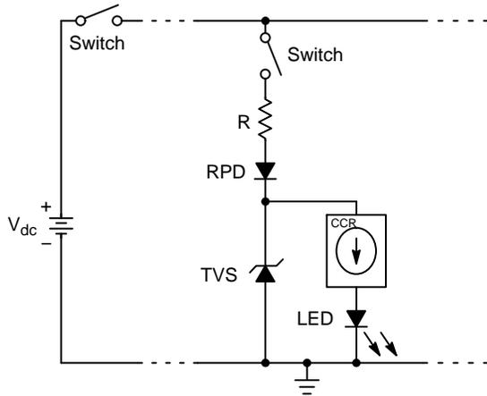
**Figure 8. CCR + LED String in Protective Network.
