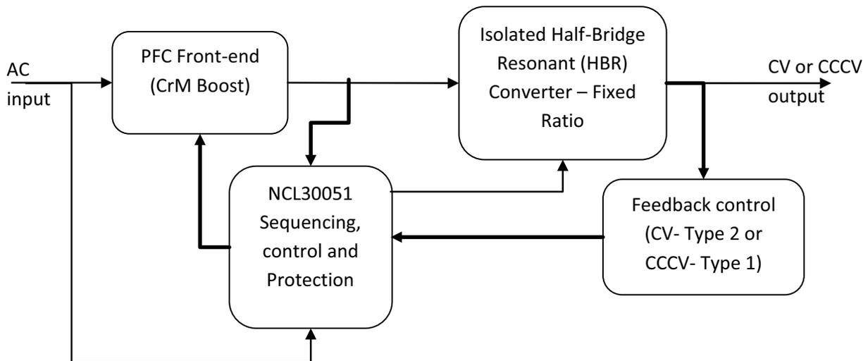
Figure 4. Simplified Control Scheme Offered by NCL30051
