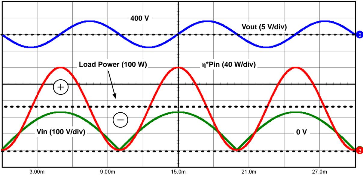
Figure 5. Relationship Between PFC Output Ripple and Input Voltage
