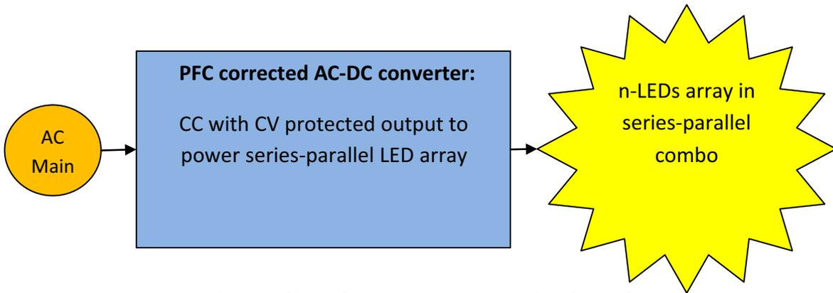
Figure 1. Single Stage Integrated LED Driver (Type 1)
