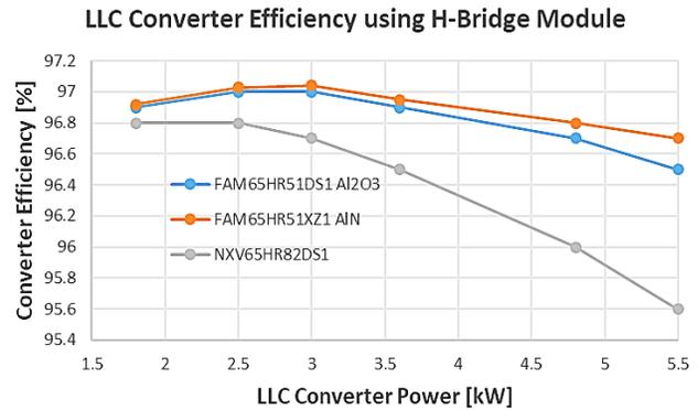
Figure 31. LLC Converter Efficiency Using H-bridge Module ( $T_{case} = 100^{\circ}C$ )
