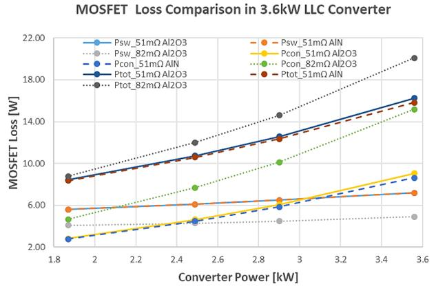
Figure 30. Power loss Comparison between 51 mΩ Die and 82 mΩ Die in H-bridge Module ( $T_{case} = 100^{\circ}C$ )
