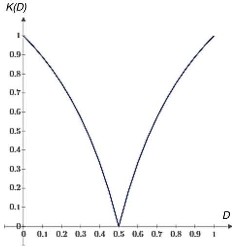
Figure 7. Ripple Reduction in PFC Boost Inductor Current by Interleaving (Ripple is Minimized at D = 0.5)
