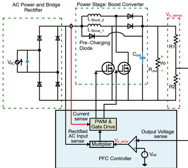
**Figure 8. Closed-loop PFC Function Block**
