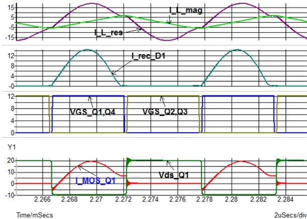
**Figure 21. Waveforms in LLC Full-bridge Converter in ZVS Region 2 ( $f_{sw} = 90 \text{ kHz}$ ,  $f_{resonant} = 100 \text{ kHz}$ )**
