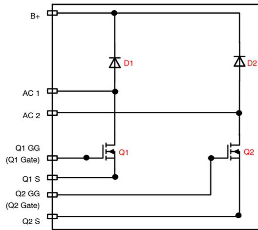
**Figure 9. Internal Circuit Diagram of FAM65CR51DZ1 PFC Module**
