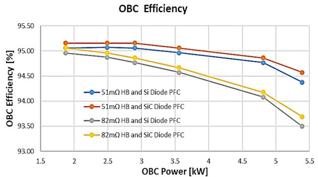
**Figure 33. OBC System efficiency by combining PFC module and H-bridge module (T<sub>case</sub> = 100°C)**
