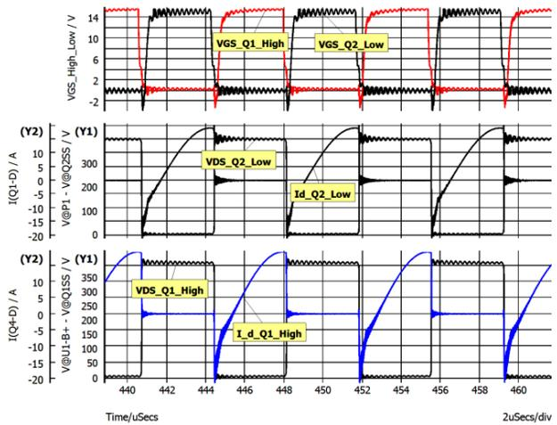
Figure 26. MOSFET Switching Waveforms in LLC Converter with 150 nF Snubber Capacitor
