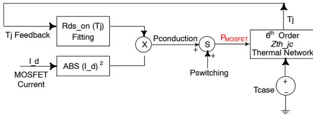
Figure 29. Thermal Analysis Block Diagram
