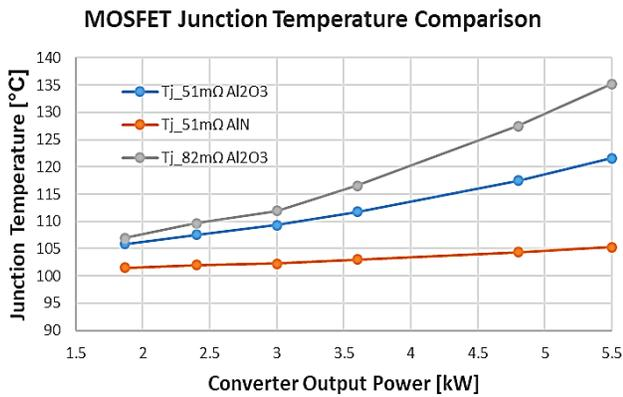
**Figure 32. MOSFET Junction Temperature Comparison in H-bridge Module (LLC Converter: T<sub>case</sub> = 100°C)**
