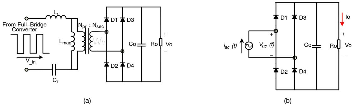
Figure 13. (a) Simplified LLC Circuit and (b) Equivalent Model Replacing Primary Side with AC Current Source
