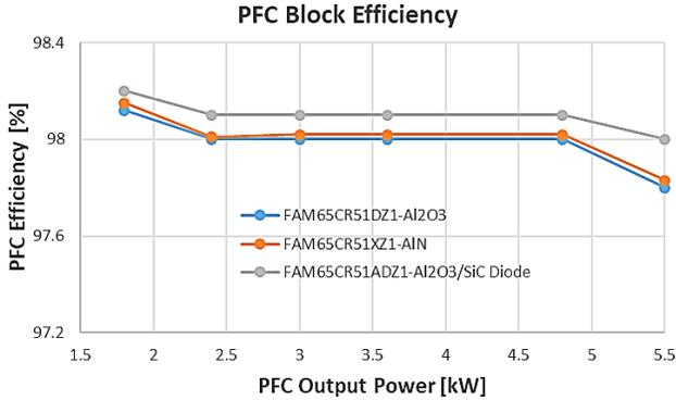
Figure 27. PFC Function Block Efficiency ( $T_{case} = 100^{\circ}C$ )
