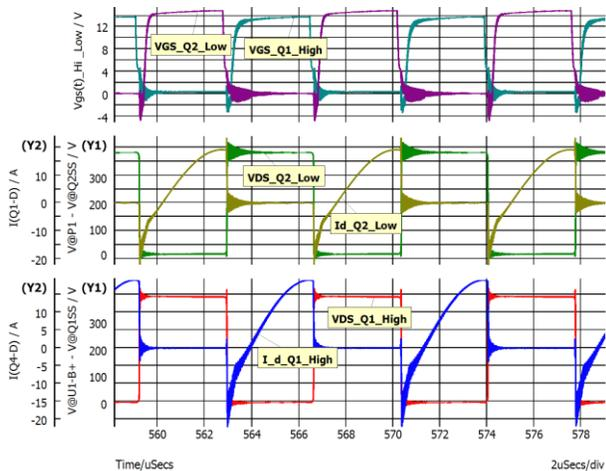
Figure 25. MOSFET Switching Waveforms in LLC Converter without Snubber Capacitor
