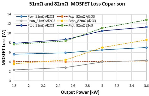
Figure 23. Power Loss Comparison between 51m and 82m Die in H-bridge Module ( $T_{case} = 100^{\circ}C$  Fixed)
