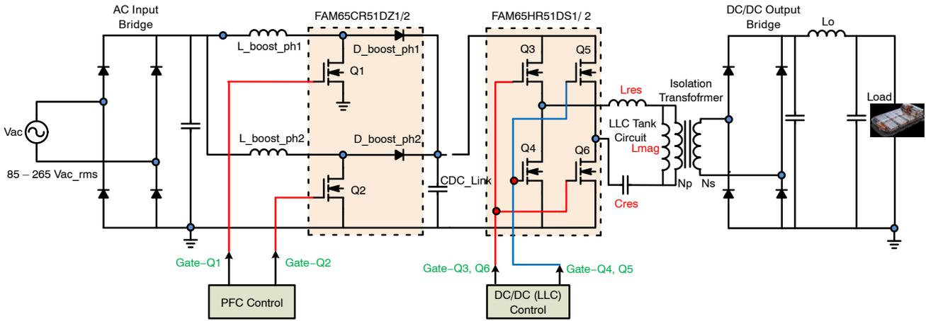
Figure 2. Block Diagram of Conventional OBC System Including Two-phase Interleaved PFC and LLC Converter
