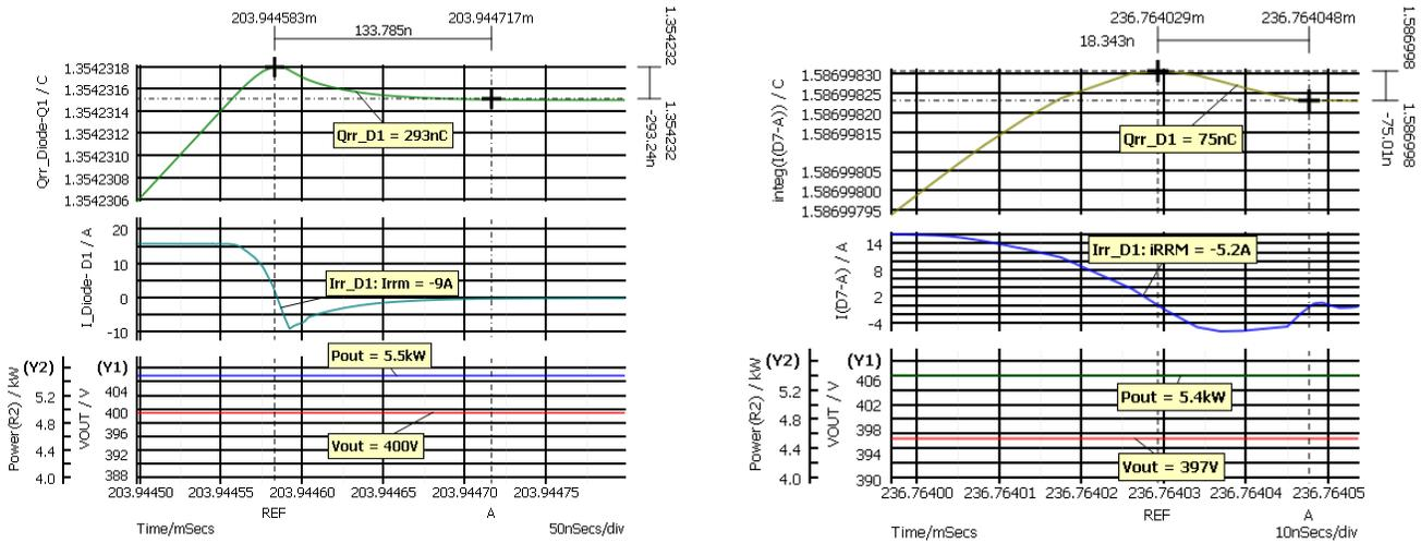
Figure 10. Reverse Recovery in ISL9R1560-F085 Stealth Diode and FFSP3065-F085 SiC Diode
