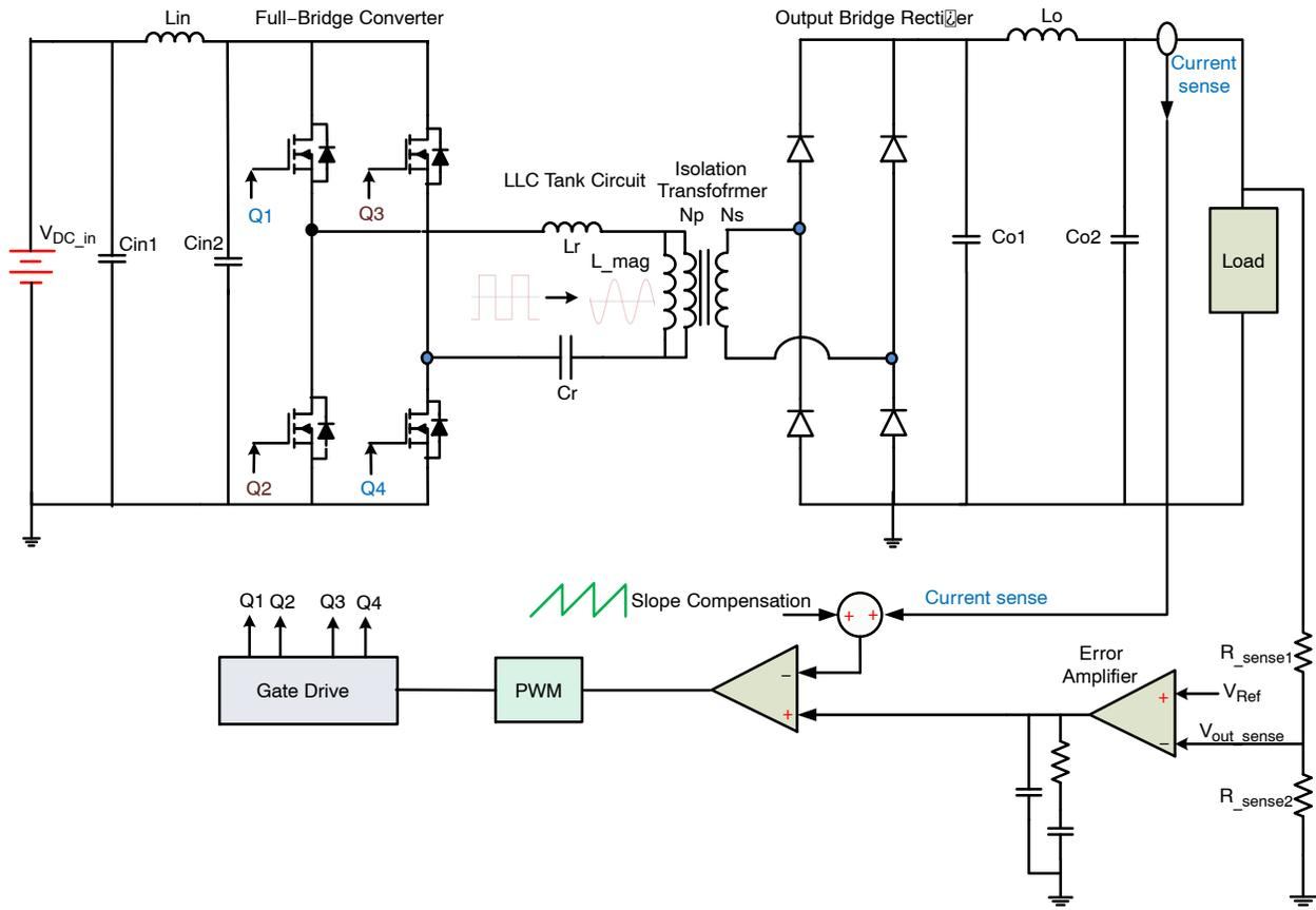
Figure 12. Full-Bridge LLC Converter Circuit with Current Mode Control
