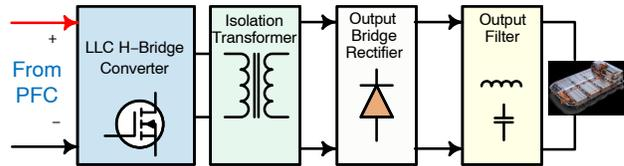
Figure 11. OBC DC/DC Converter Block Diagram
