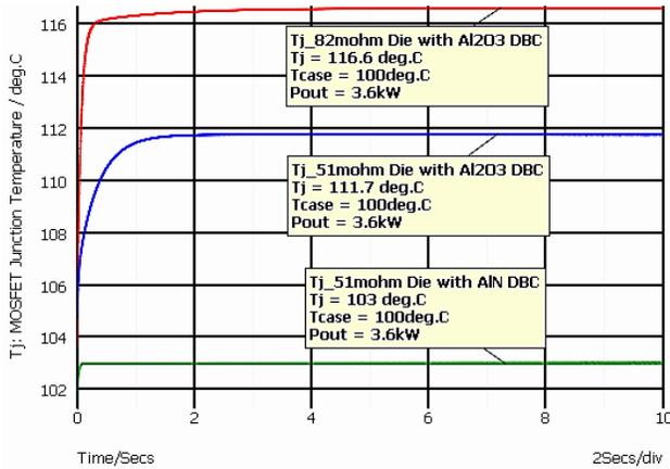
Figure 24. Junction Temperature Comparison between 51m and 82m Die in 3.6 kW LLC Converter ( $T_{case} = 100^{\circ}C$  Fixed)
