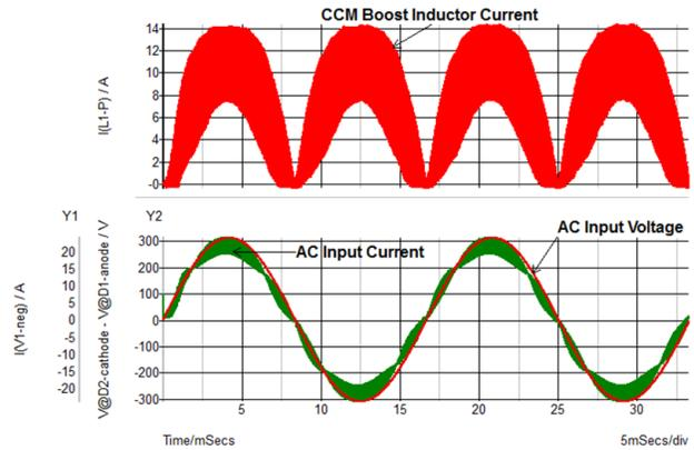
Figure 3. Phase Matching between Input Voltage and Current in a CCM PFC
