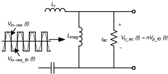
Figure 14. AC Equivalent Circuit for LLC Resonant Converter
