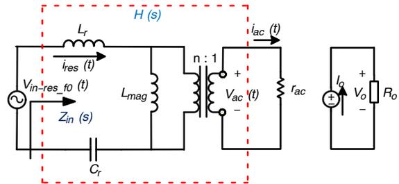
Figure 15. Two Port Network Model of FHA Resonant Circuit
