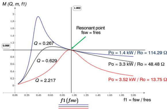
Figure 16. LLC Converter Gain Variation in Accordance with the Load Shift
