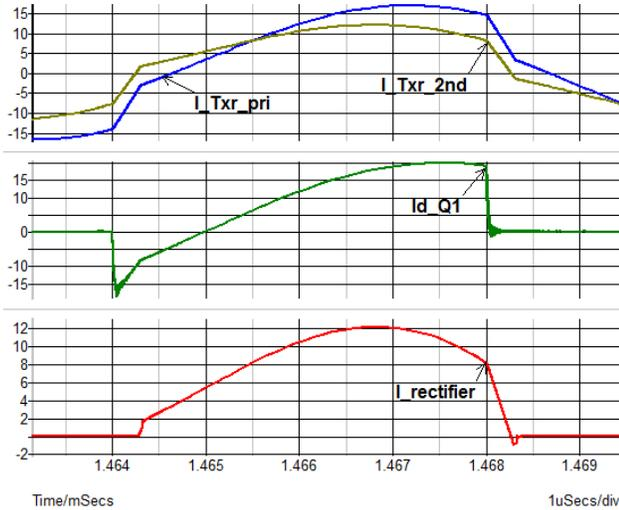
**Figure 20. Secondary Side Rectifier Diode Hard Commutation During the MOSFET Turn-off Transient**
