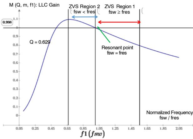
Figure 17. LLC Converter Gain Graph at 3.3 kW Load Condition
