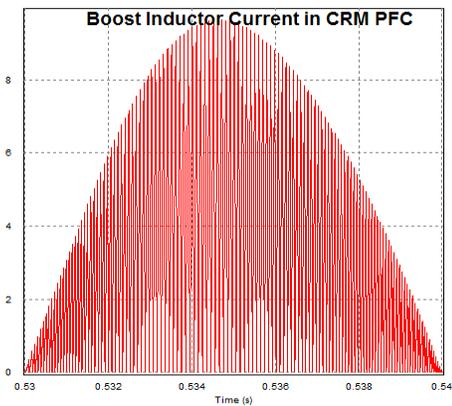
Figure 4. Boost inductor current in CRM PFC
