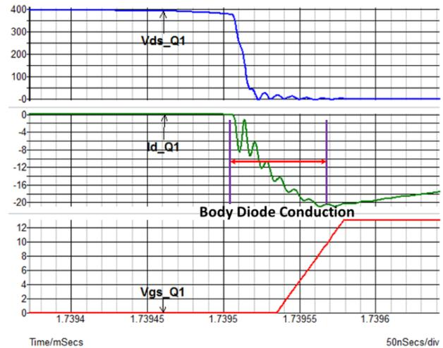
Figure 19. ZVS Operation: Gate Drive Signal is Engaged During the Body Diode Conduction ( $V_{ds} \approx 0 \text{ V}$ )
