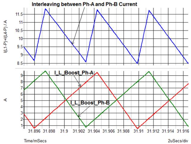
Figure 6. Current Ripple Reduction in Two-phase Interleaved Boost PFC Circuit
