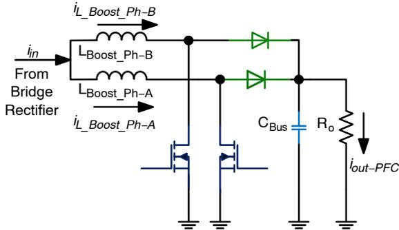
Figure 5. Interleaving of Two-phase Current
