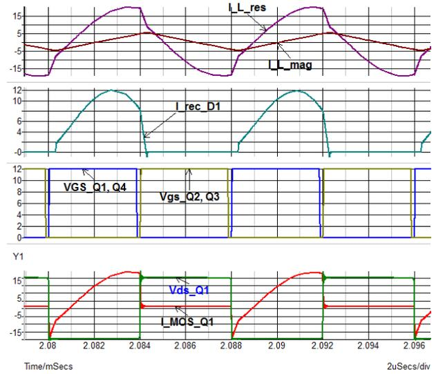
Figure 18. Typical Waveforms in LLC Full-bridge Converter ( $f_{sw} = 125 \text{ kHz}$ ,  $f_{res} = 100 \text{ kHz}$ )
