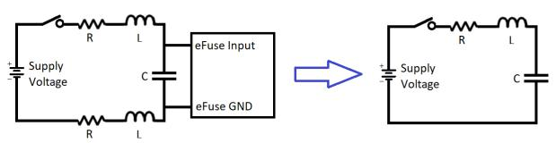
Figure 3. The System Schematic is Converted to a Simplified Series RLC Circuit since the eFuse can be Considered High Impedance. Also since the Positive and GND Return Cables are in Series they can be Lumped Together
