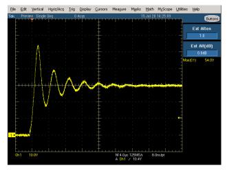
Figure 9. Lab Measurement with 1 µF Capacitor and an NIS5420 eFuse Connected in Parallel
