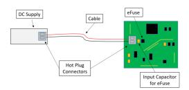
Figure 2. System Diagram
