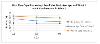
Figure 10. R vs. Average Max Capacitor Voltage
