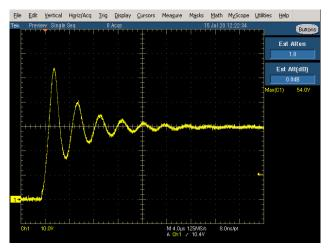
Figure 8. Lab Measurement Hot Plugging into a 1 μF Capacitor Only (no eFuse)
