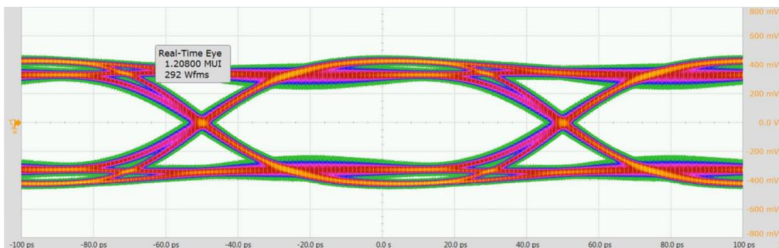
Figure 11. Eye Diagram Using Negative Flat Gain
