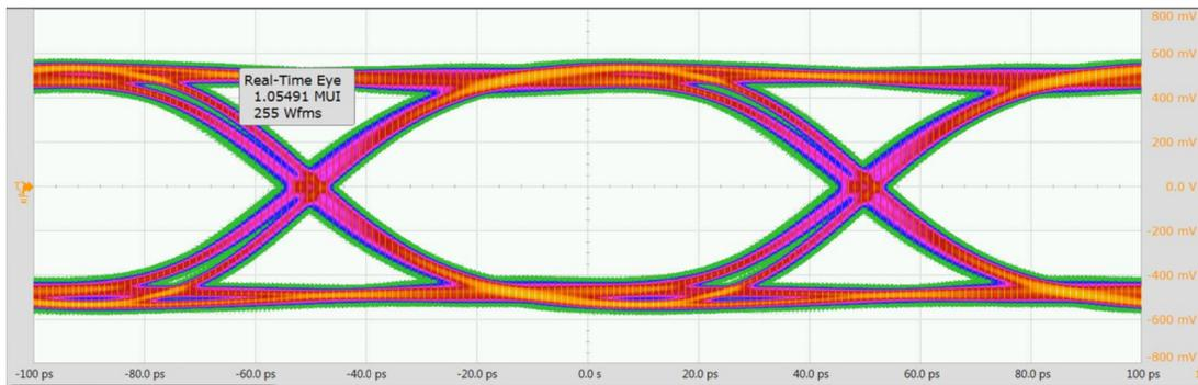
Figure 9. Eye Diagram Using Correct Equalization
