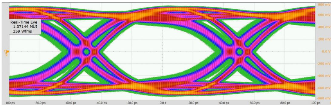
Figure 14. Eye Diagram with Distortion from Driving Signal Past Compression Point
