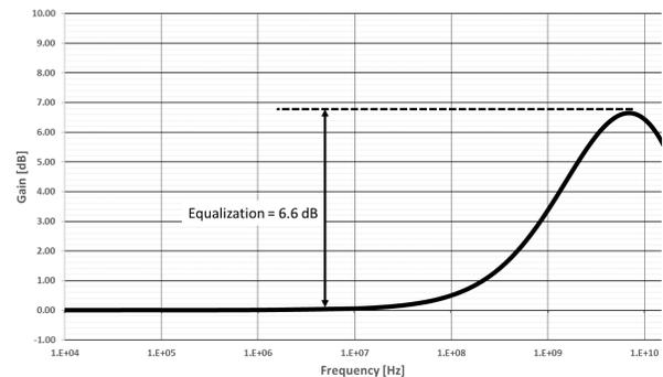
Figure 1. Equalization Gain Plot across Frequency
