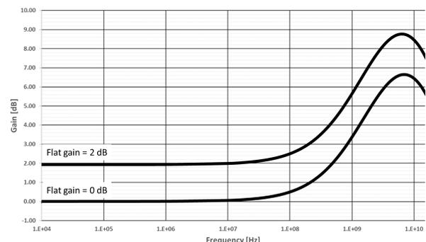
Figure 2. Flat Gain Plot across Frequency
