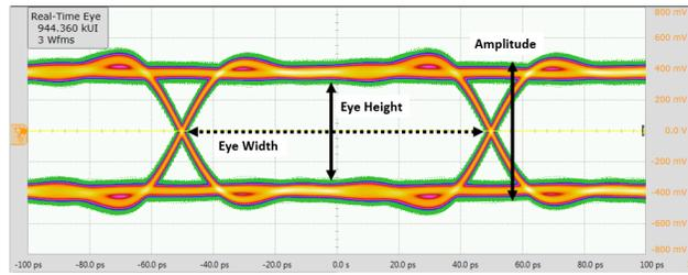
Figure 4. Eye Diagram Key Measurements
