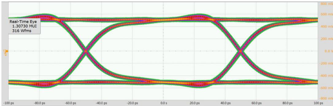
Figure 6. Eye Diagram of Signal before Loss
