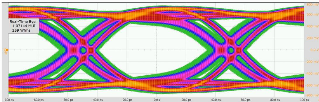
Figure 10. Eye Diagram Using Too Much Equalization
