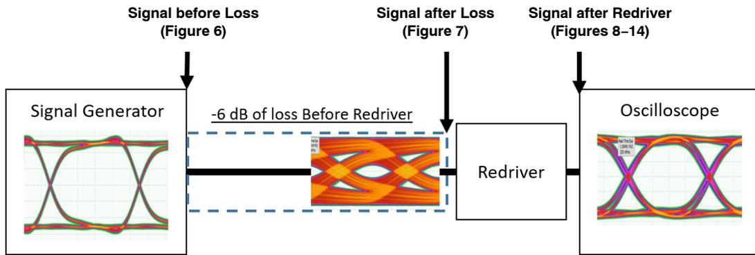
Figure 5. Block Diagram and Location of Signals
