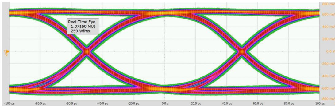
Figure 13. Eye Diagram Using Positive Flat Gain
