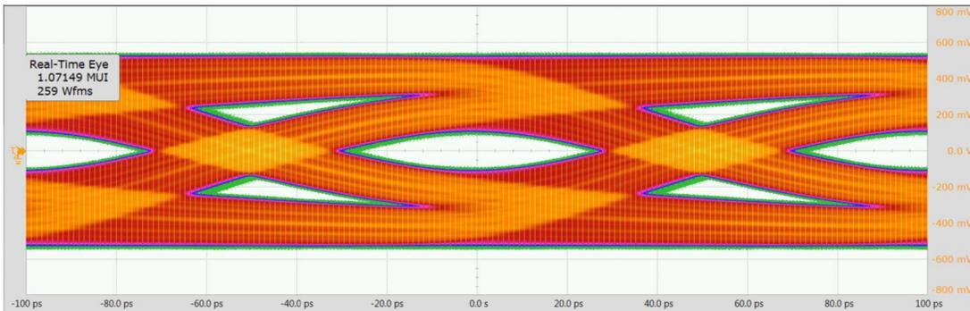
Figure 7. Eye Diagram of Signal after Loss
