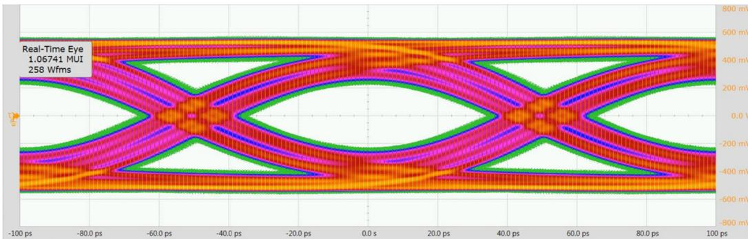
Figure 8. Eye Diagram Using Too Low of Equalization
