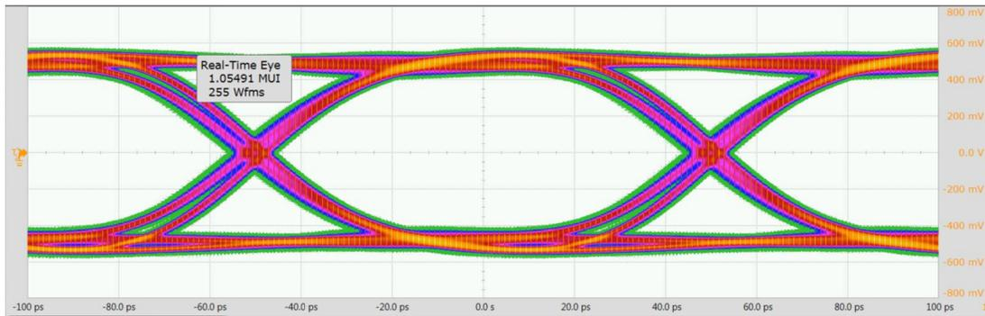
Figure 12. Eye Diagram Using No Flat Gain
