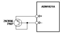
Figure 2. Connections for Discrete NPN and PNP Transistors
