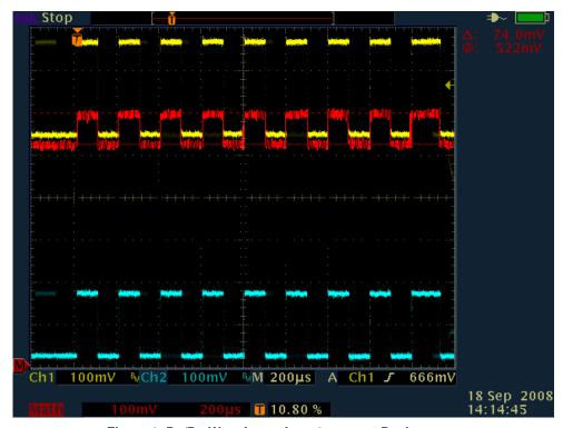
Figure 3. D+/D- Waveforms for a 2-current Device
