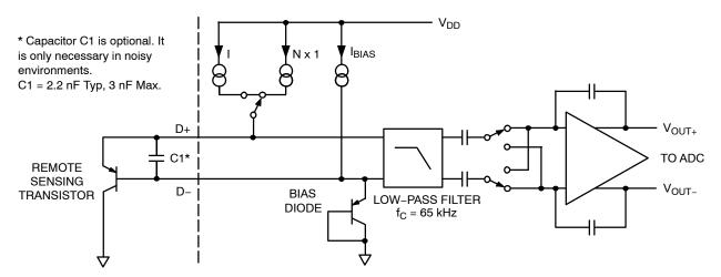
Figure 1. Internal Circuit for 2-current Device
