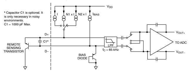
Figure 7. Internal Circuit for 3-current Device
