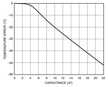
Figure 6. Temperature Error due to D+/D- Capacitance
