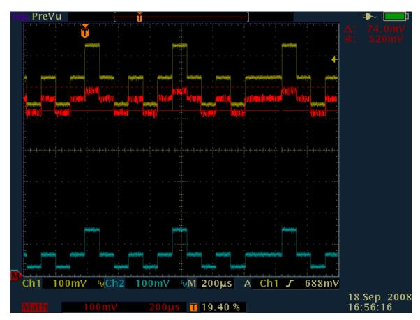
Figure 8. Typical D+/D- Waveforms for 3-current Device
