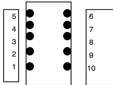
Figure 3. Bobbin Pinout - Bottom View
