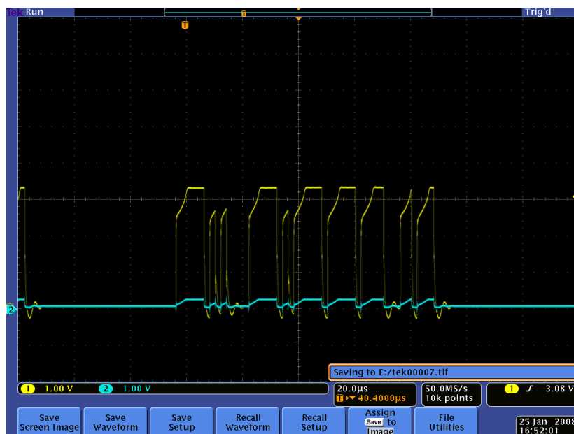
Figure 7. Data Frame Periodically Sent by the HS-CAN Node when CANL is Shorted to Ground – Yellow Trace = CANH; Blue Trace = CANL
